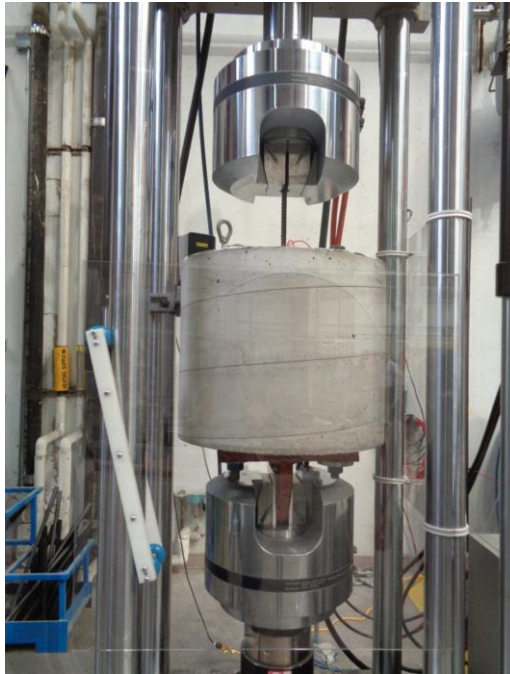
Figure 2.4 Test setup for (a) pullout and (b) shear tests (Shrestha et al. 2017)
