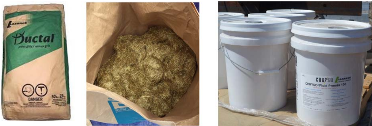
Figure 4-6 Ductal® UHPC mixture components: (a) dry Ductal® premix; (b) steel fibers; and (c) superplasticizer.
