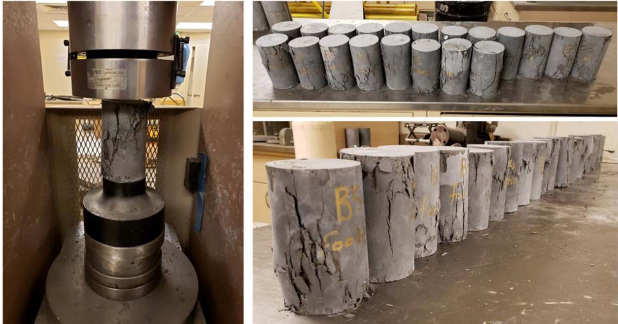
Figure 4-12 UHPC cylinder damage and mode of failure under compression tests.
