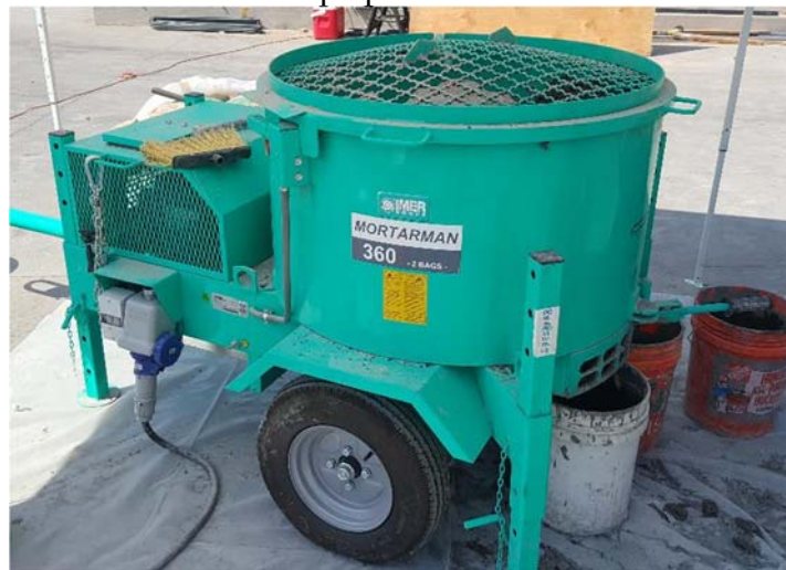
Figure 4-7 UHPC high shear mixer at UNR (Imer 750).
