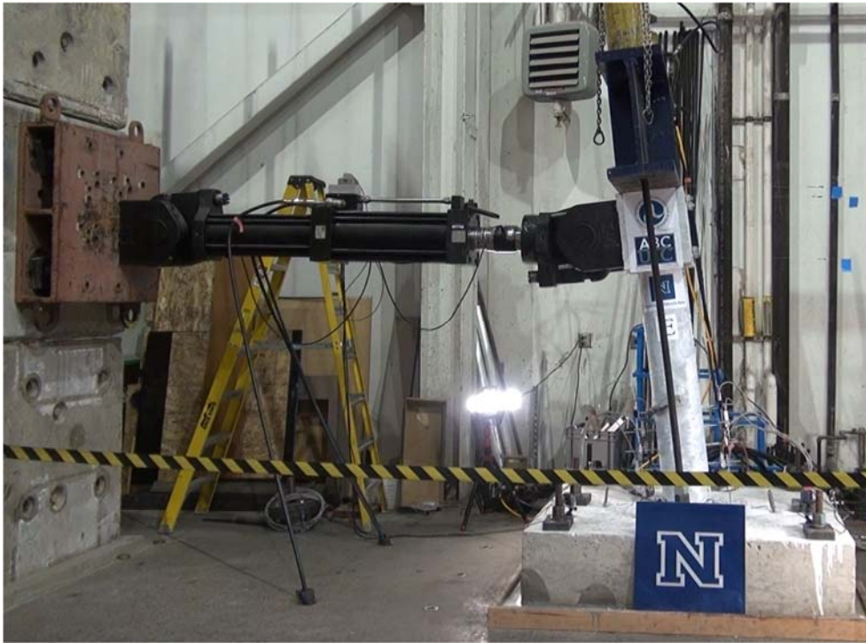
Figure 5-1 Overview of Column Model Under Maximum Drift.
