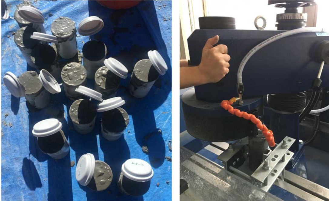
Figure 3-2 Fresh UHPC after filling the cylinders (left) and process of grinding the cylinders ends for straight and smooth surface for compression testing (right).
