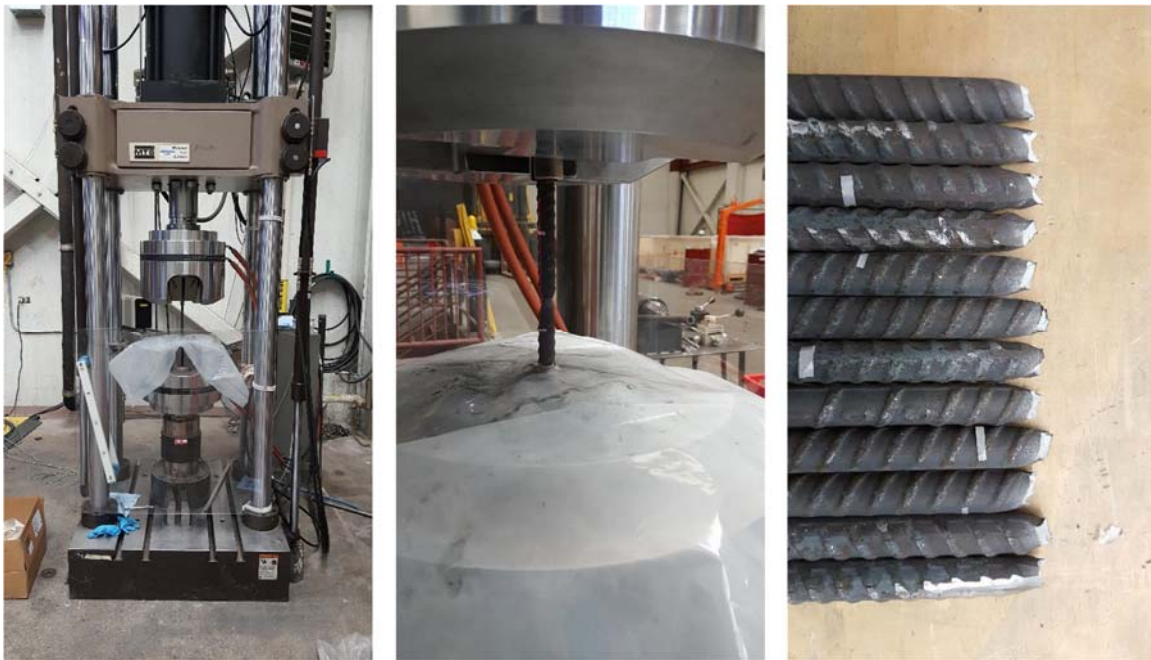
Figure 4-15 Direct tension tests on #5 rebar samples.
