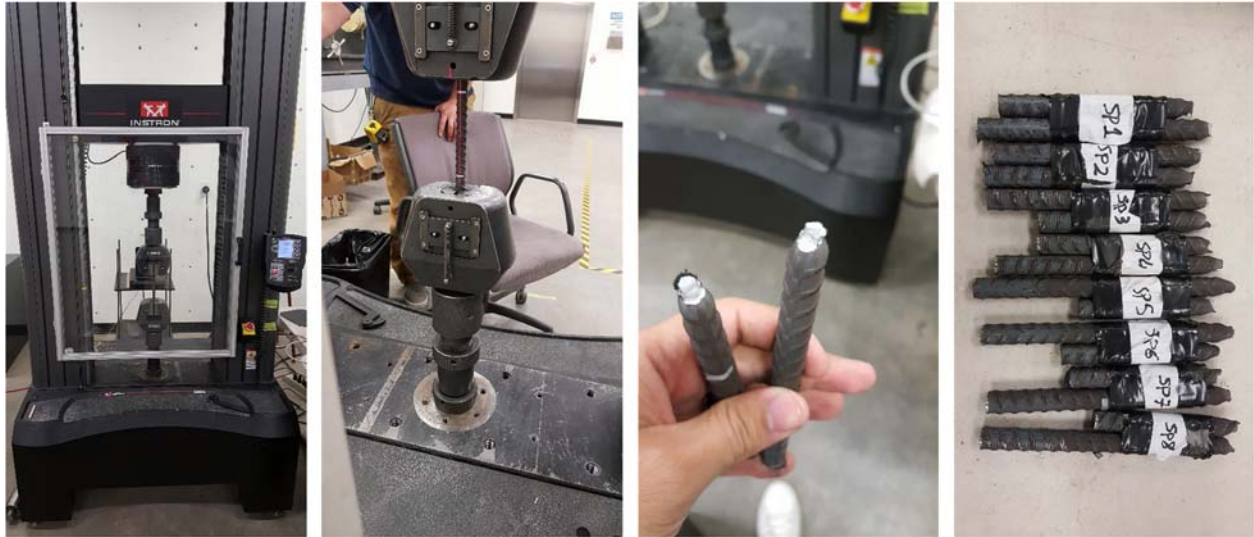
Figure 4-14 Direct tension tests on #4 rebar samples.
