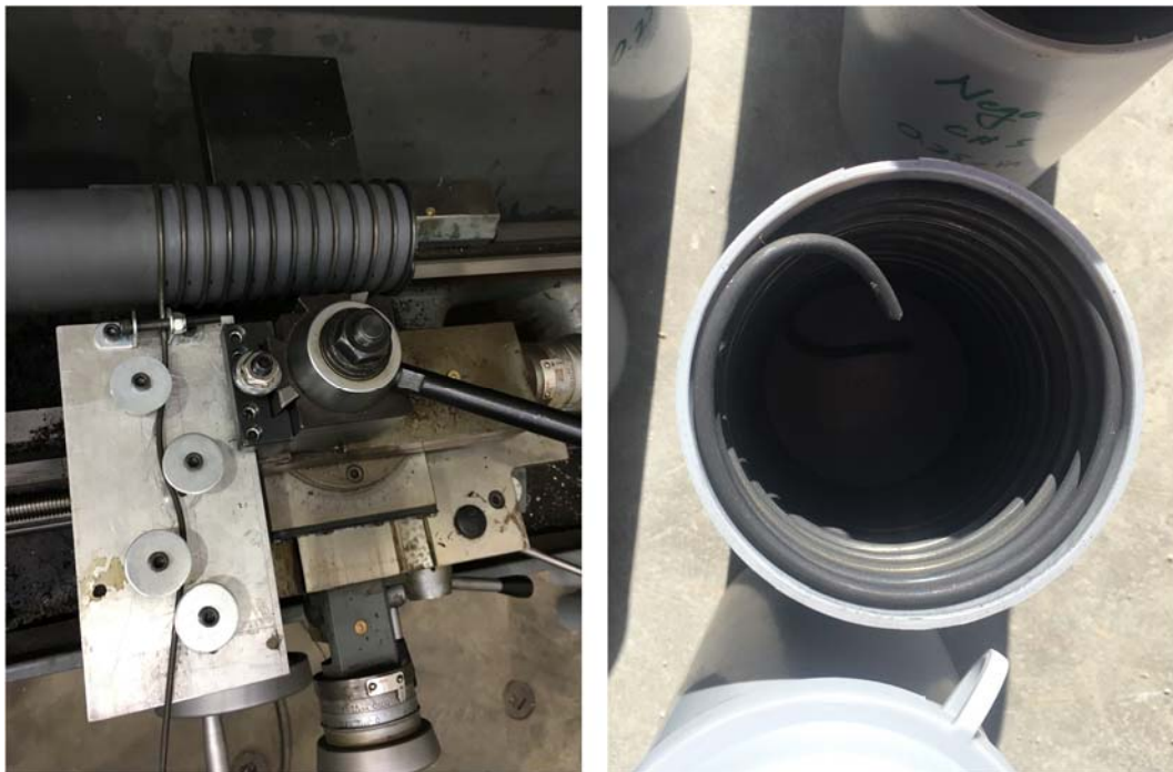
Figure 3-1 Assembling the spirals used for the UHPC confinement study.
