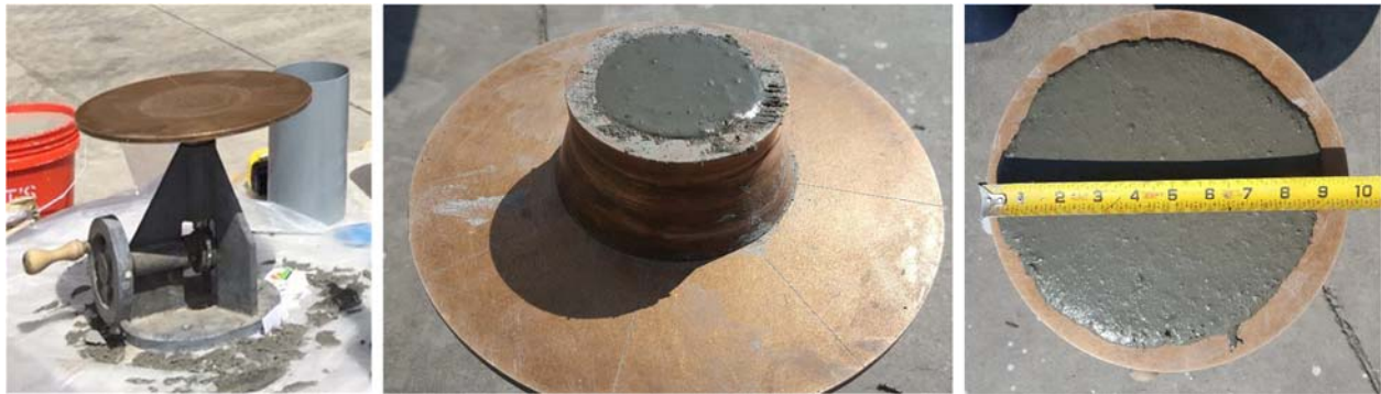
Figure 4-9 UHPC slump testing.
