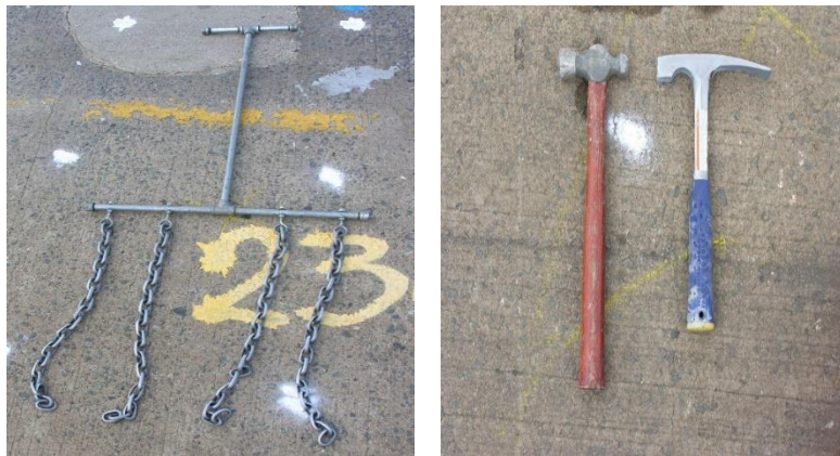
Figure 1. Chain drag equipment (left) and hammer sounding tools (right)
