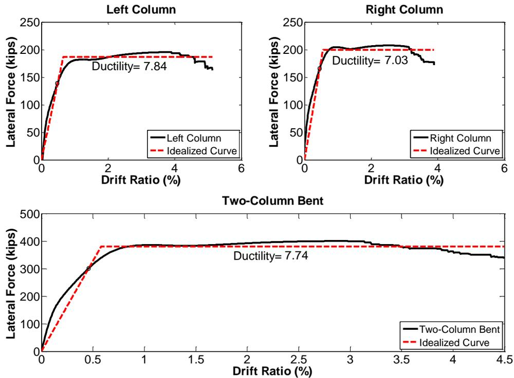
Figure 2-2. Pushover Response of Reference Bent for Loading from Left
