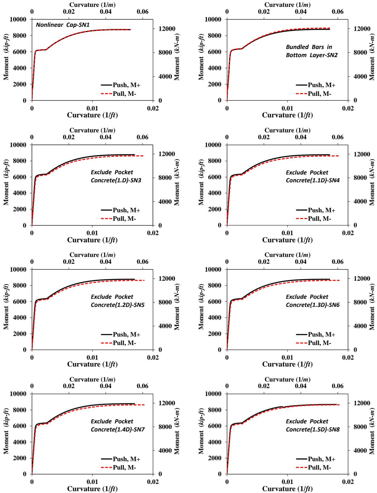
Figure 2-6. Moment-Curvature Relationships for Reference Cap Beam
