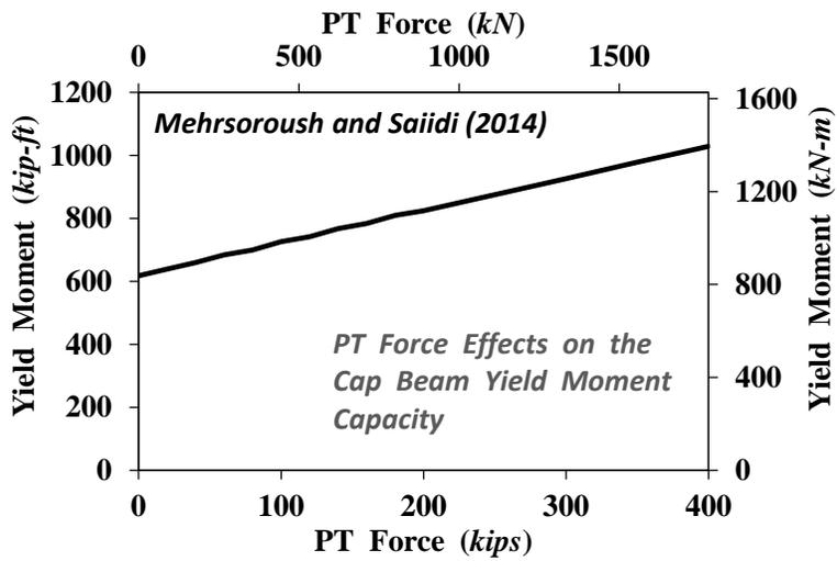
Figure 2-13. Post-tensioning Force Effects on Cap Beam Yield Moment Capacity
