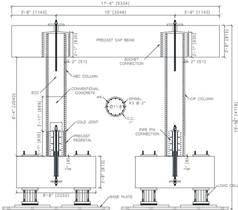
(a) Two-Column Bent with Precast Cap Beam
