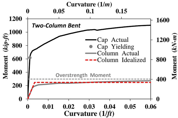
Figure 2-12. Moment-Curvature Relationships for Bent Tested by Mehrsoroush and Saiidi (2014)
