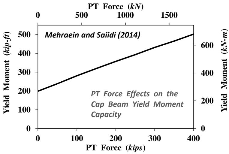
Figure 2-15. Post-tensioning Force Effects on Cap Beam Yield Moment Capacity
