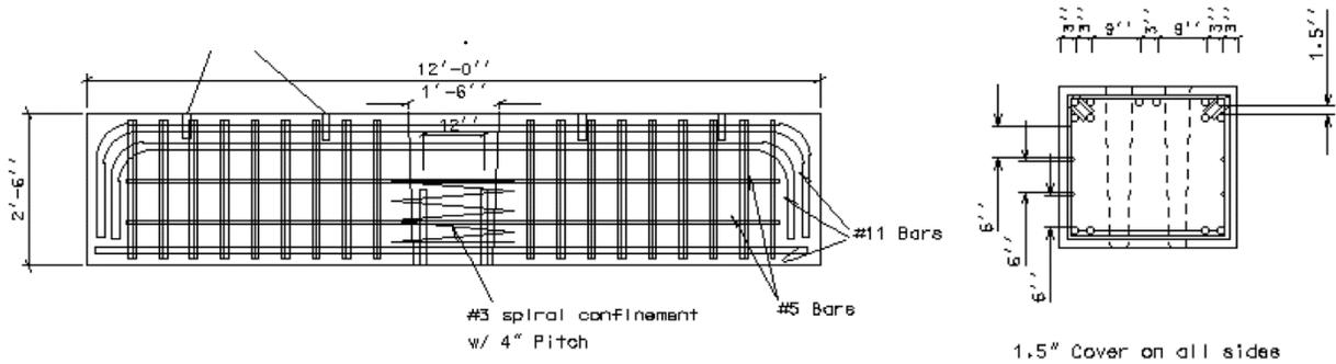
(b) Cap Beam Elevation View
