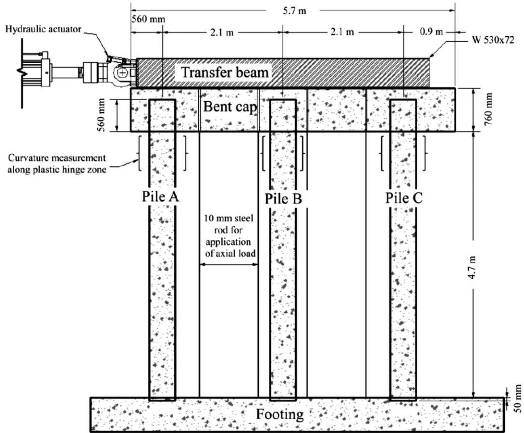
(a) Pile to Cap Specimen (Larosche et al., 2014b)
