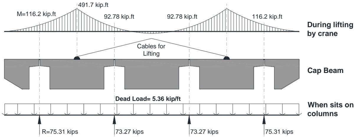
**Figure 5-2. Bent Cap Moment and Punching Forces during Lifting and Installing**
