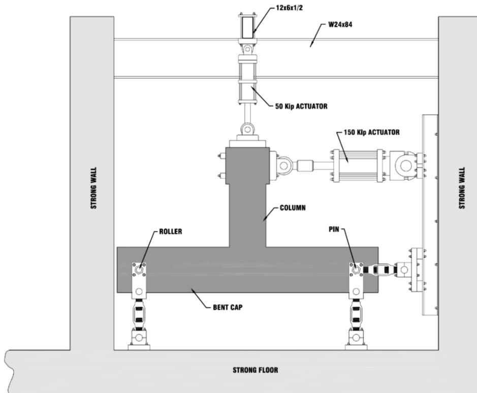
Figure 2-10. Cap Beam Pocket Connection Test Setup (Restrepo et al., 2011)
