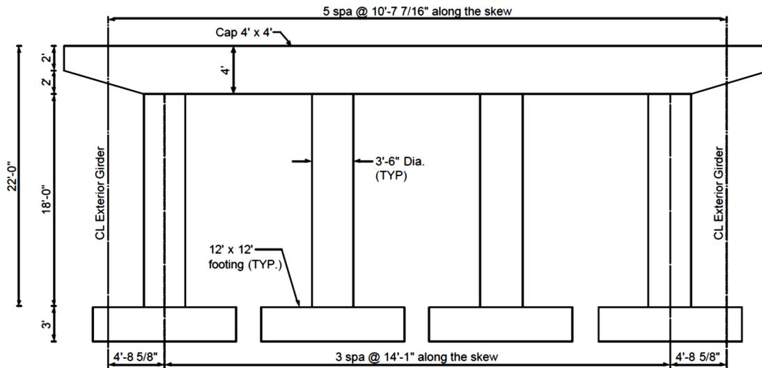
(b) Bent Elevation
