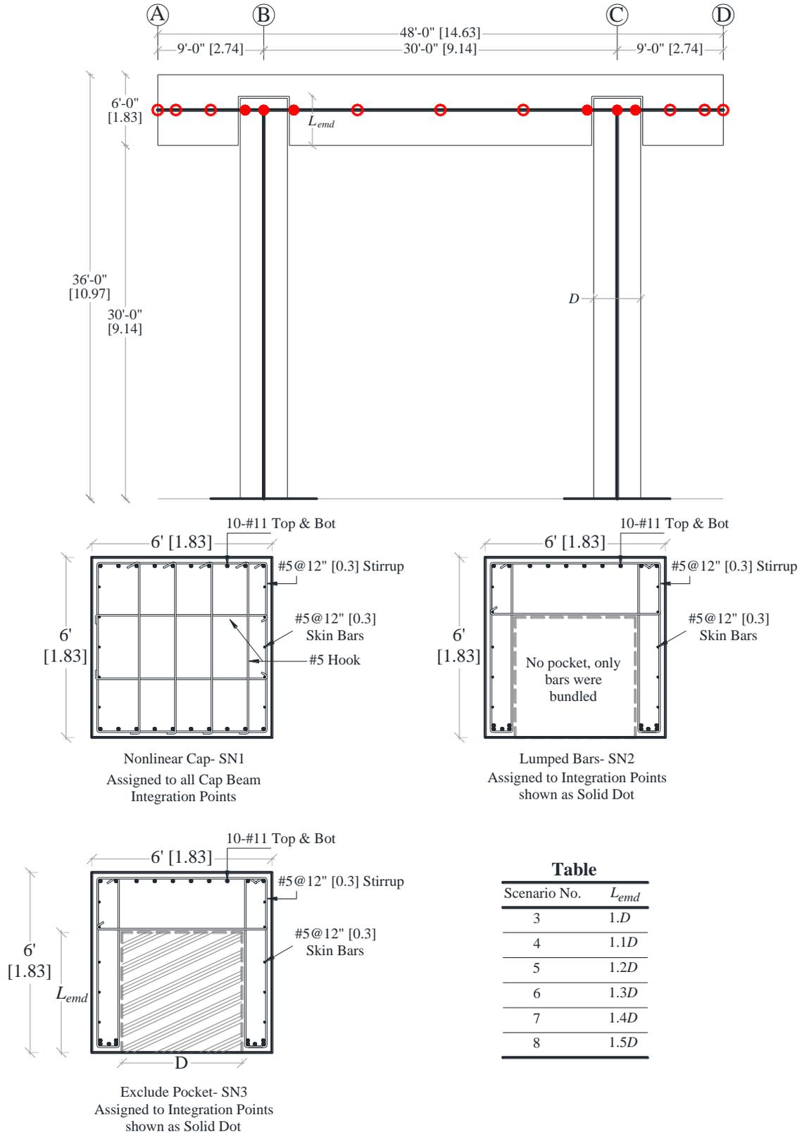
**Figure 2-5. Different Scenarios for Bent with Pocket Connections, units: ft [m]**
