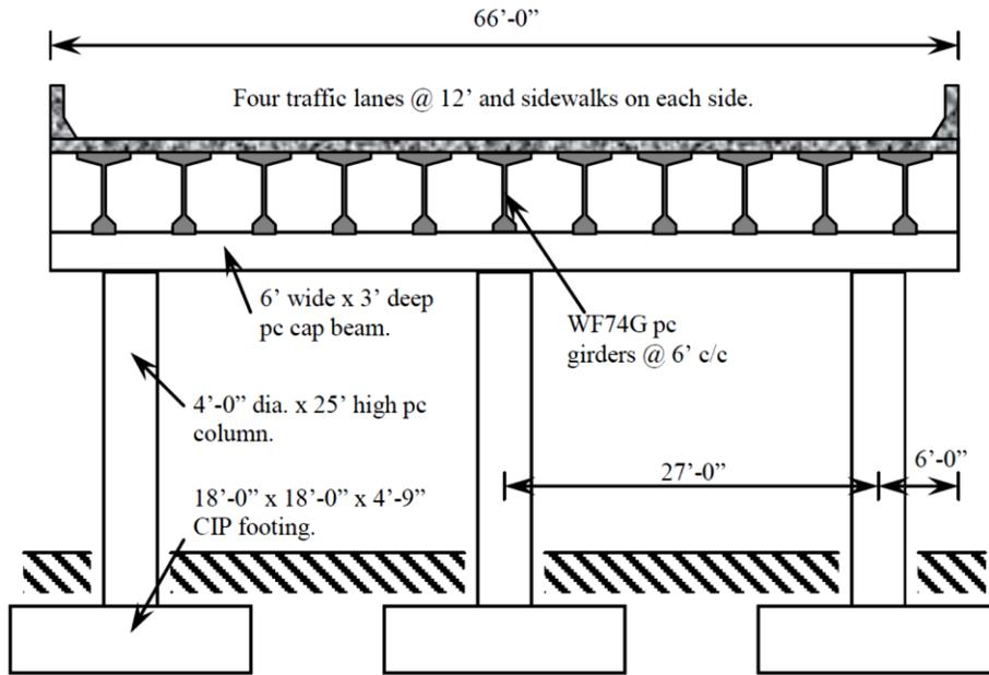
**Figure 3-2. Reference Cast-in-Place Bent (Marsh et al. 2011)**
