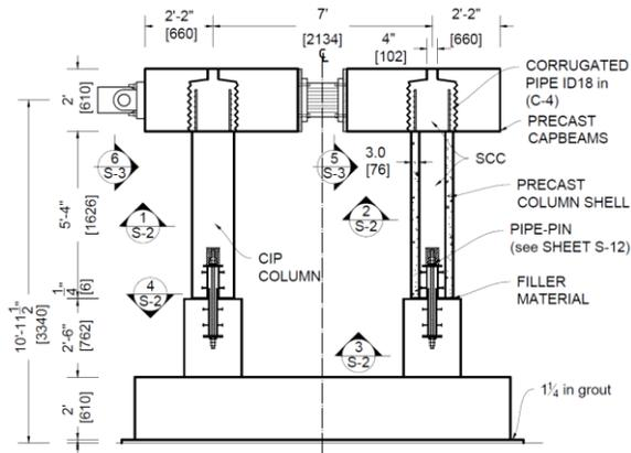
(a) Two-Column Bent with Precast Cap Beams
