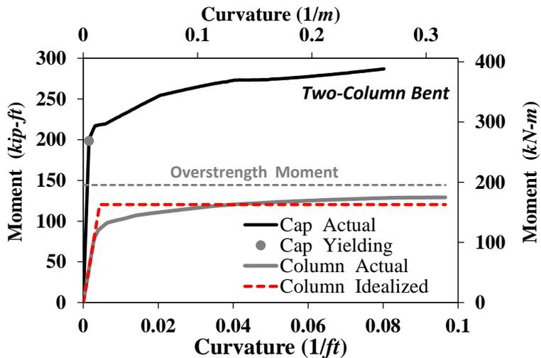
Figure 2-14. Moment-Curvature Relationships for Bent Tested by Mehraein and Saiidi (2014)
