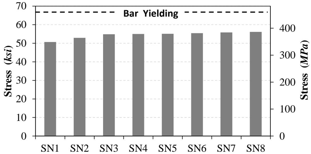
Figure 2-9. Peak Tensile Strains of Cap Beam Steel Bars for Different Scenarios
