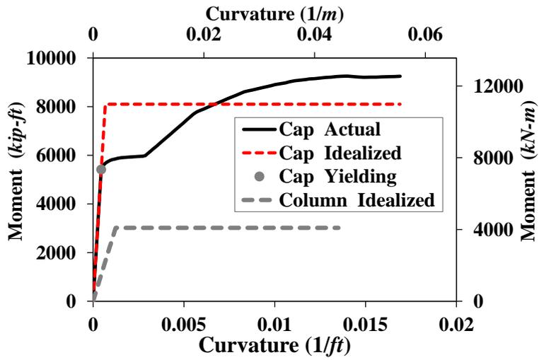
Figure 2-3. Moment-Curvature Relationships for Reference Bent Cap Beam and Columns
