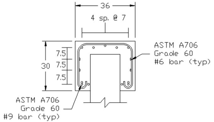
(c) Bent Cap Section at the center-line of Pile C (Cukrov and Sanders, 2012)
