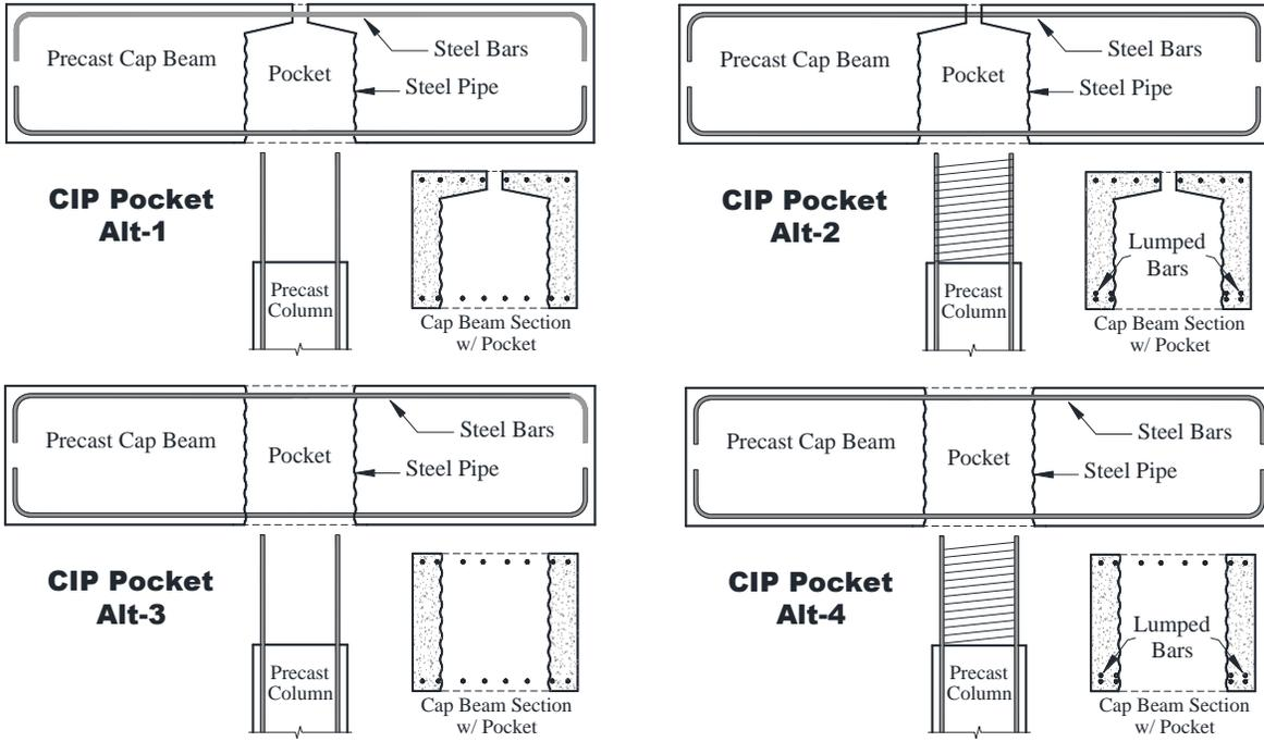
(a) Cast-in-Place Pocket Connections
