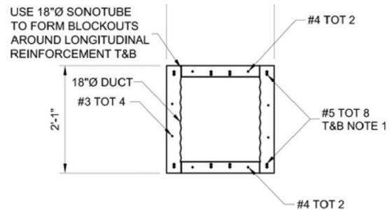
(c) Cap Beam Elevation (Left) and Section B (Right) for CPLD
