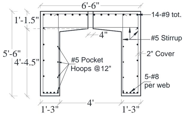
(c) Cap Beam Section with Pocket
