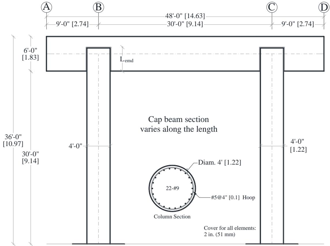
Figure 2-4. Reference Two-Column Bent Details with Pocket Connections, units: *ft* [*m*]
