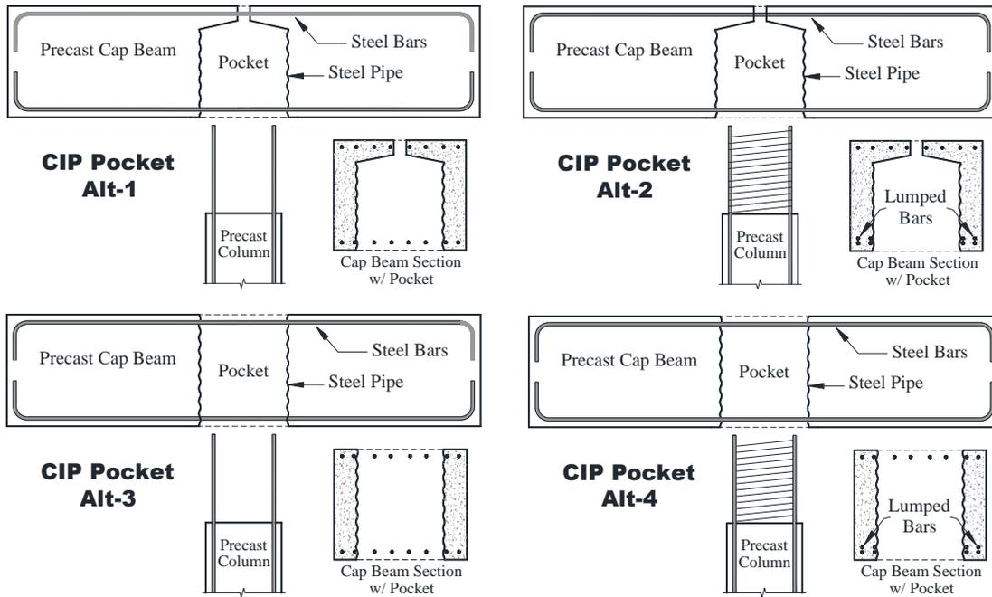
(a) Cast-in-Place Pocket Connections
