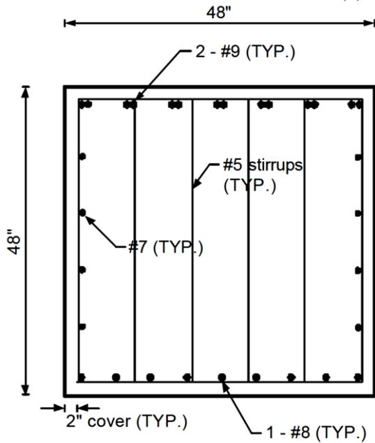
(c) Cap Beam Section
