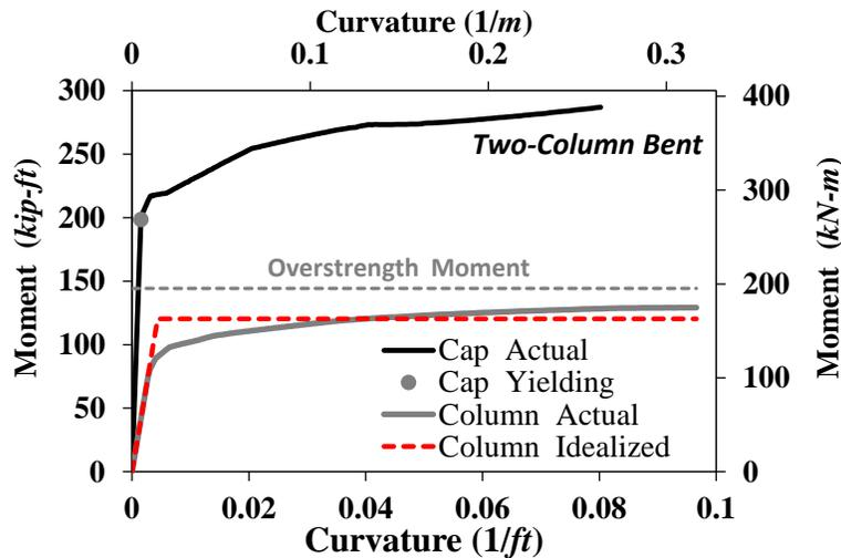
**Figure ES-2. Moment-Curvature Relationships for Bent Tested by Mehraein and Saiidi (2014)**
