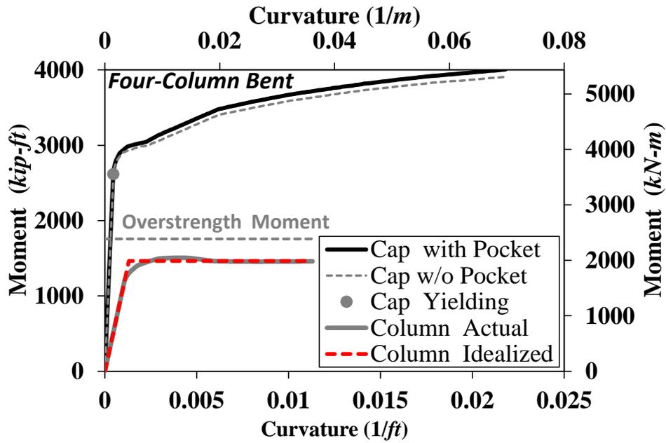
Figure 5-4. Precast Bent Cap Moment-Curvature Relationship
