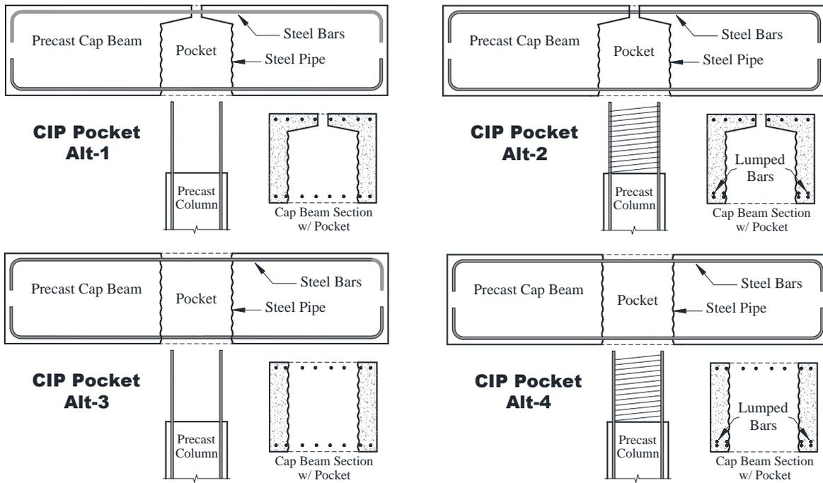
(a) Cast-in-Place Pocket Connections
