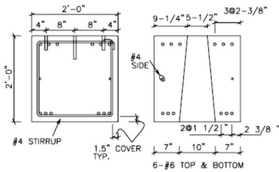
(c) Cap Beam Details for Single-Line Pocket
