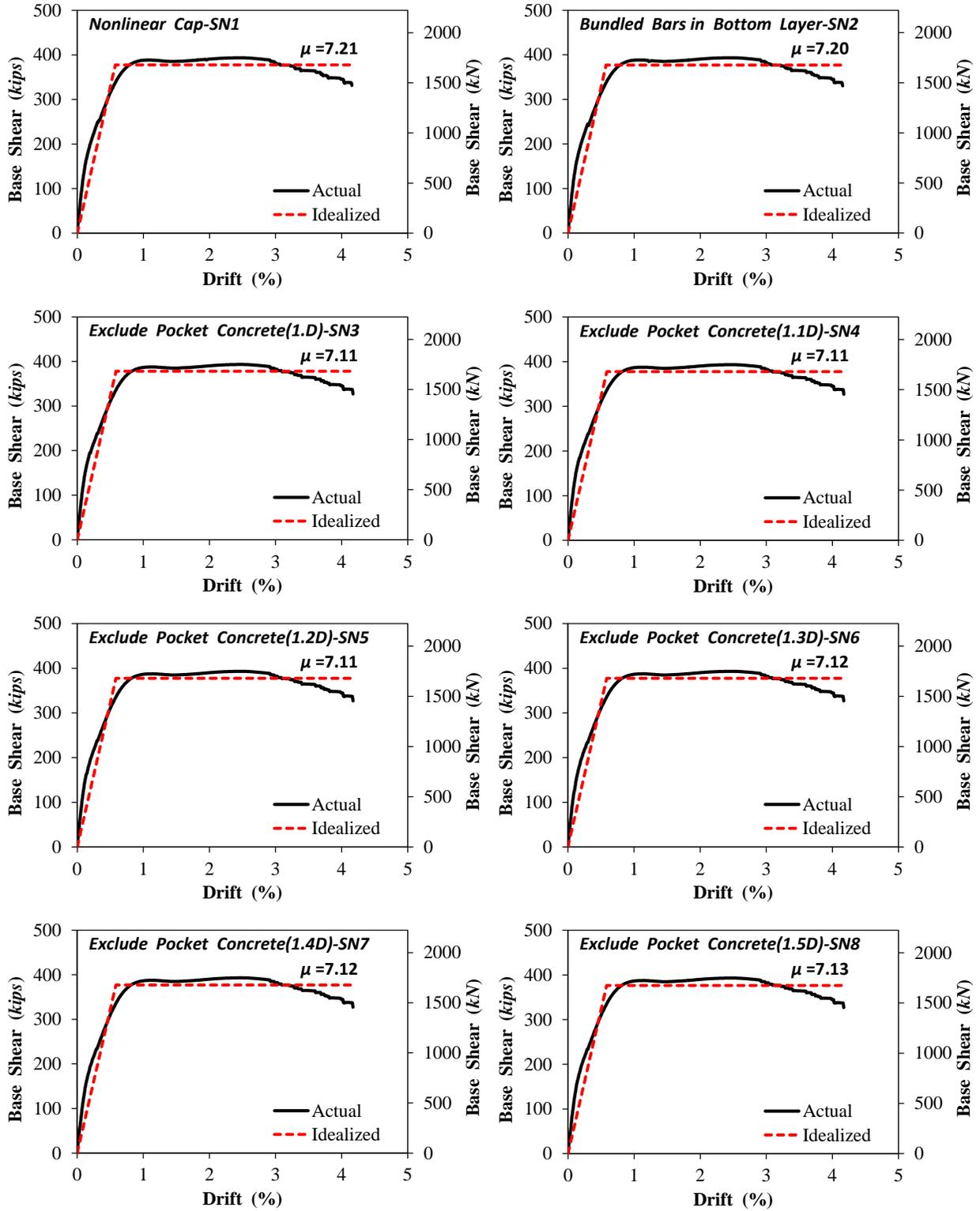
Figure 2-8. Pushover Curves for Reference Two-Column Bent
