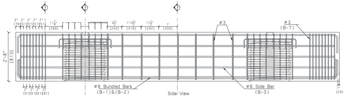
(b) Cap Beam Elevation
