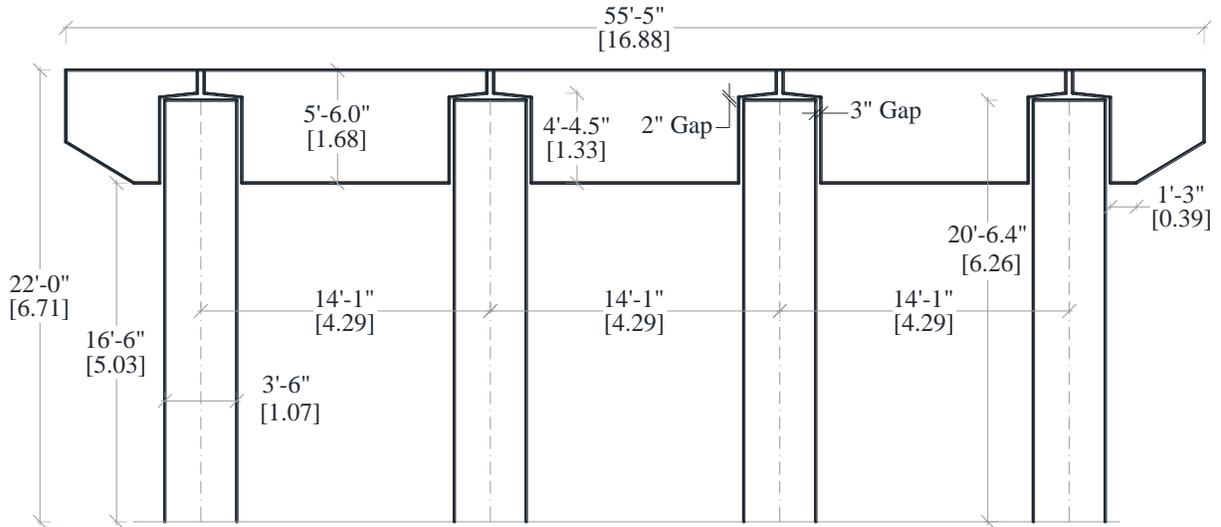
(a) Bent Elevation
