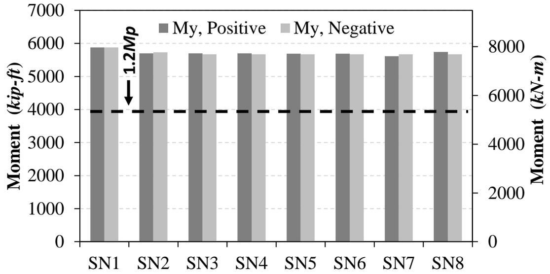
Figure 2-7. First Yield Moment for Reference Cap Beam for Different Scenarios
