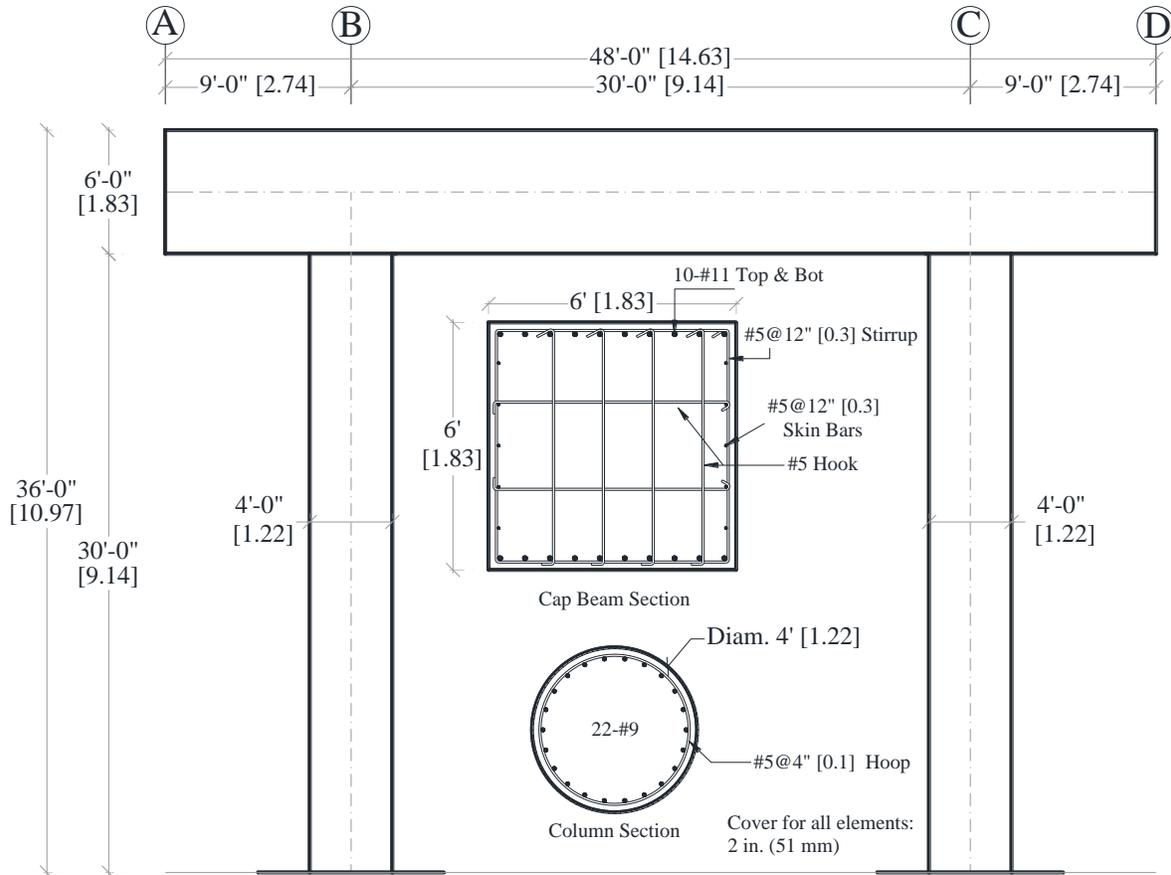
Figure 2-1. Reference Two-Column Bent Details, units: *ft [m]*
