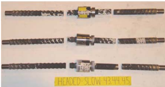
(a) Slow-Strain Rate Tests (failure shown on right-side of coupler)
