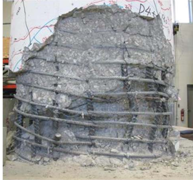
(b) Plastic Hinge of Original Column after Testing
