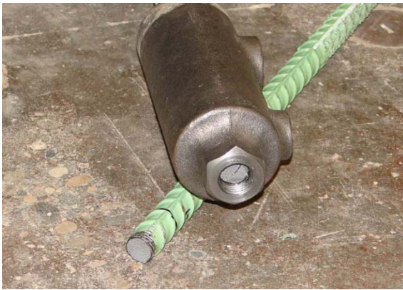
(a) Bar fracture in one of three Tests
