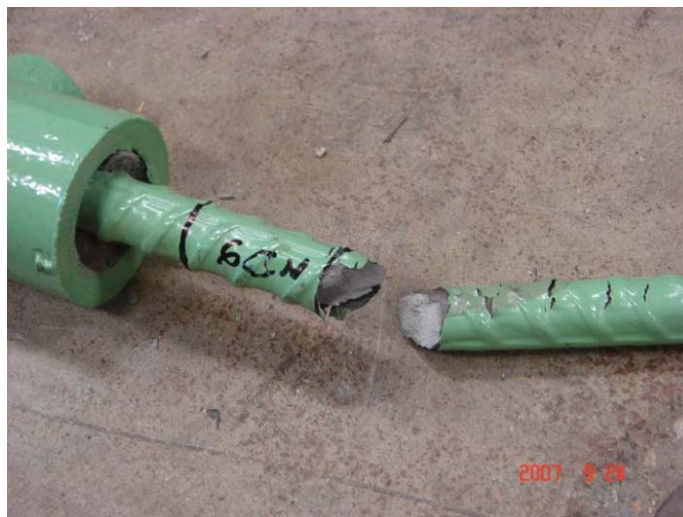
(c) Bar fracture in one of three Tests
