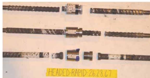
(c) Rapid-Strain Rate Tests (failure shown on right-side of coupler)
