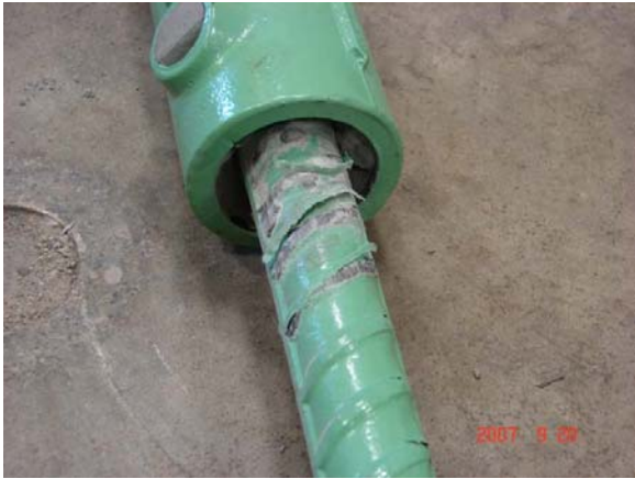
(a) Pull-out failure in one of three SSGCs
