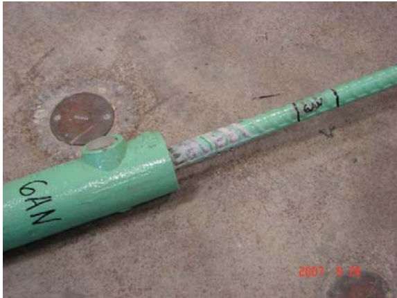
(a) Pull-out failure in one of three Tests
