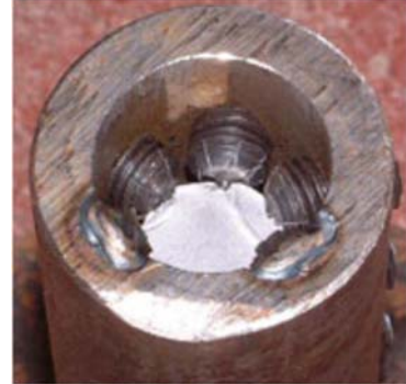
(b) Failure of SMA inside Coupler
