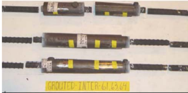
Figure 1-18. Grouted Coupler Specimen Tests under Intermediate Strain Rate (Rowell et al., 2009)
