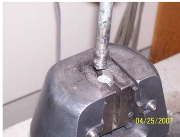
(c) SMA Failure at threads
