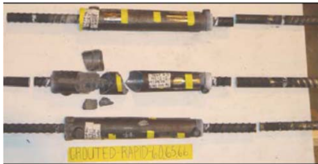
Figure 1-19. Grouted Coupler Specimen Tests under High Strain Rate (Rowell et al., 2009)
