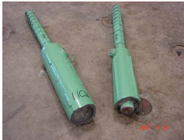
(c) Splice fracture in one of three SSGCs
