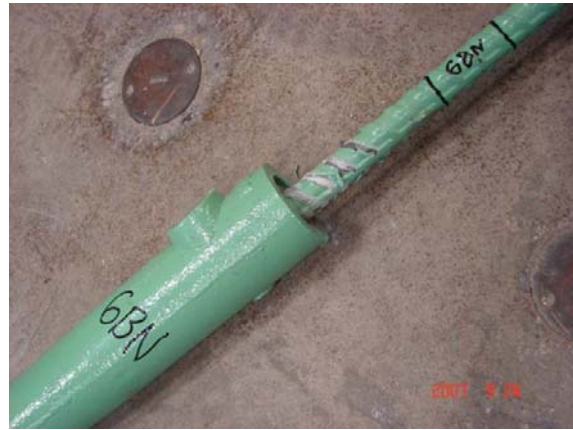
(b) Pull-out failure in one of three Tests
