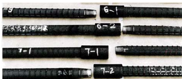
Figure 1-23. Taper Threaded Coupler Specimen Tests (Noureddine, 1996)
