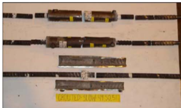
Figure 1-17. Grouted Coupler Specimen Tests under Low Strain Rate (Rowell et al., 2009)
