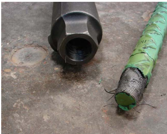
(c) Thread failure in one of three Tests
