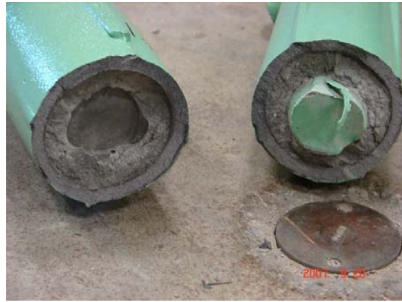
(b) Splice failure in one of three SSGCs
