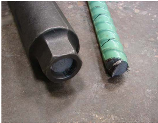
(a) Bar fracture in one of three Tests
