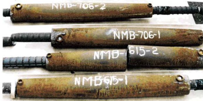
Figure 1-12. Grouted Coupler Specimen Tests (Noureddine, 1996)
