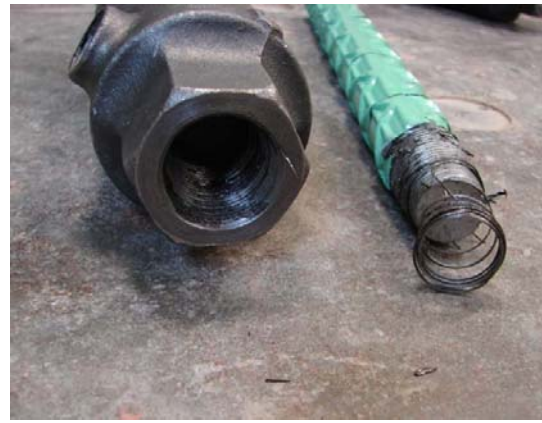
(b) Thread failure in all three Tests
