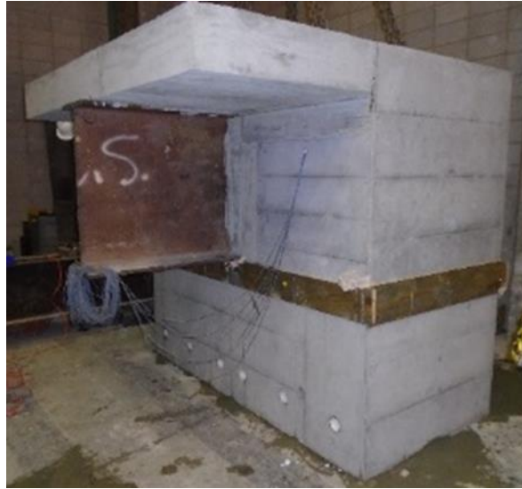
Figure 49. Grout bed formwork back
