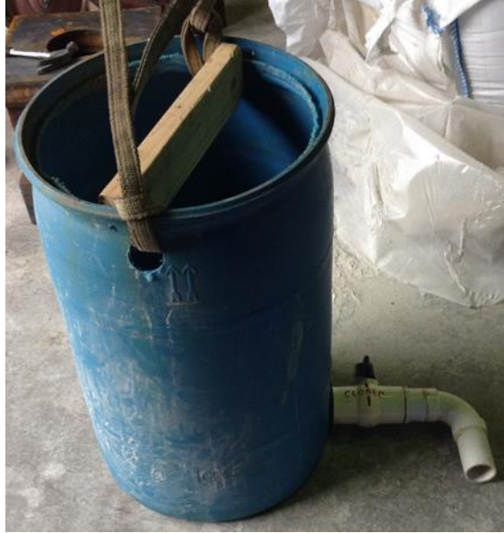
Figure 51. Grout funnel system
