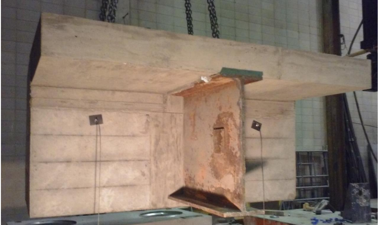
Figure 46. Integral diaphragm with suspended HP sections
