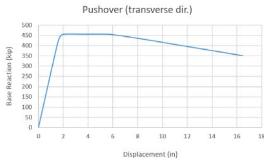
Figure 5-38 Pushover curve for the transverse direction of earthquake excitation.
