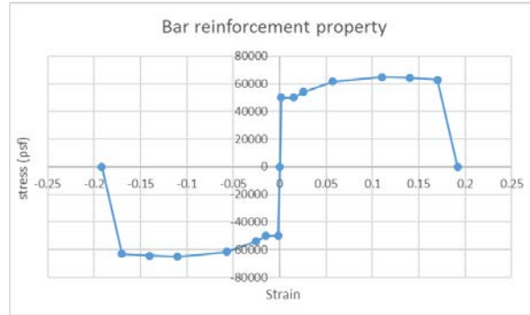
Figure 5-6 Stress-strain curve of bars.
