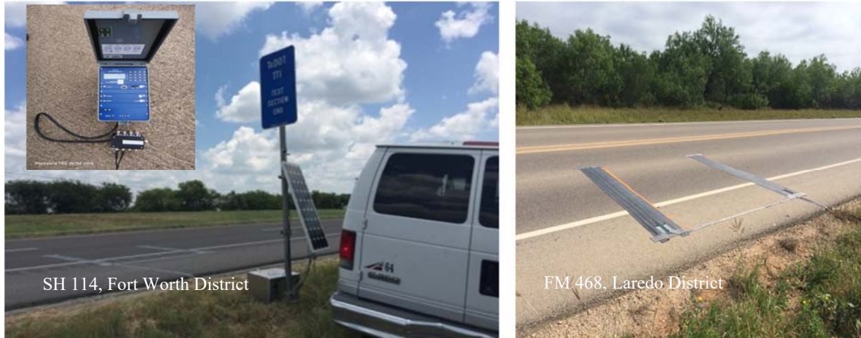
Figure 4. Portable WIM Setup—SH 114 and FM 468.
