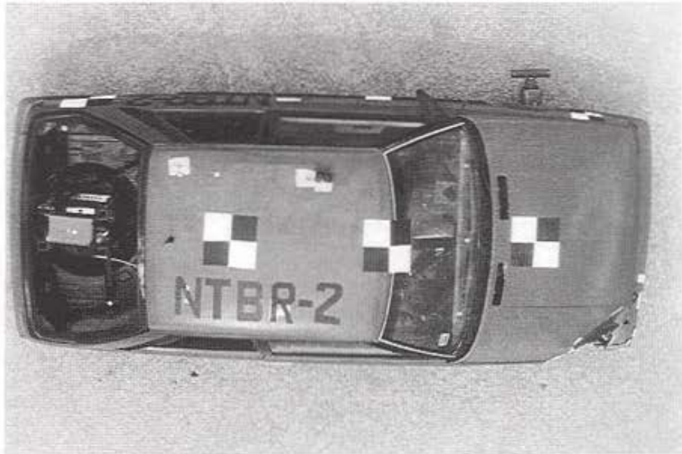
Figure 102. Vehicle Damage, Test NTBR-2.
