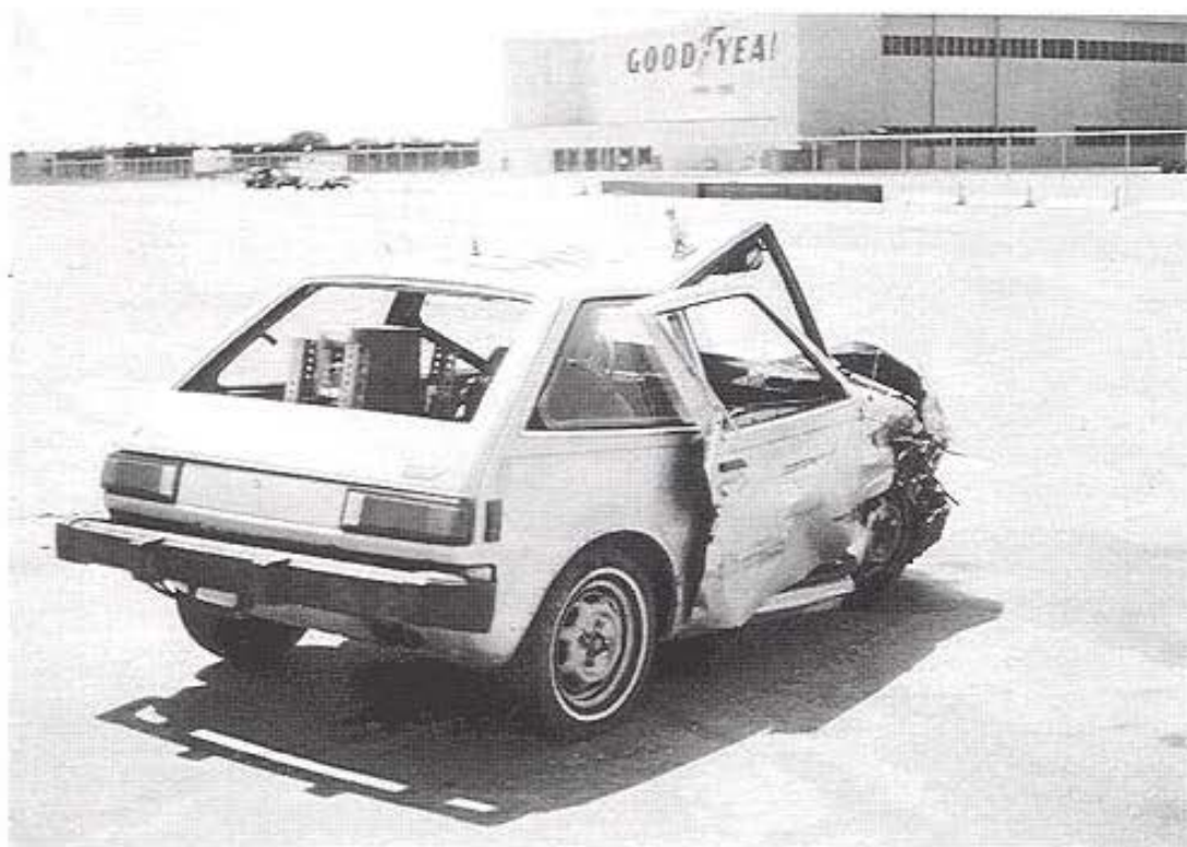
Figure 48. Vehicle Damage, Test GWMP-1.
