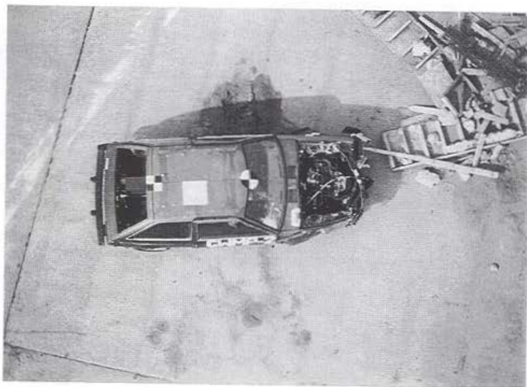
Figure 54. Vehicle Damage, Test GWMP-2 (continued).
