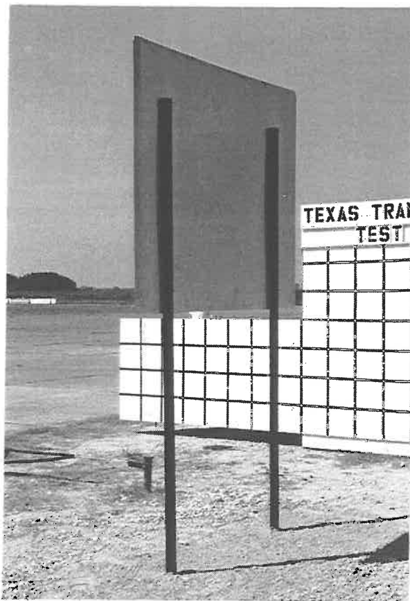
Figure 76. Dual 2-1/2 lb steel U-channel support installation anchored in strong soil before test 405231-11.
