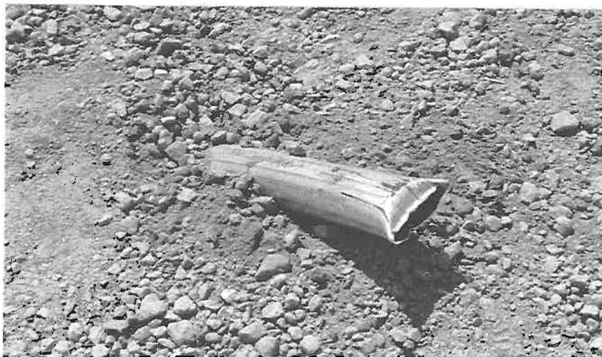
Figure 45 . Single 4 in. aluminum sign support installation anchored in strong soil after test 405231-6.
