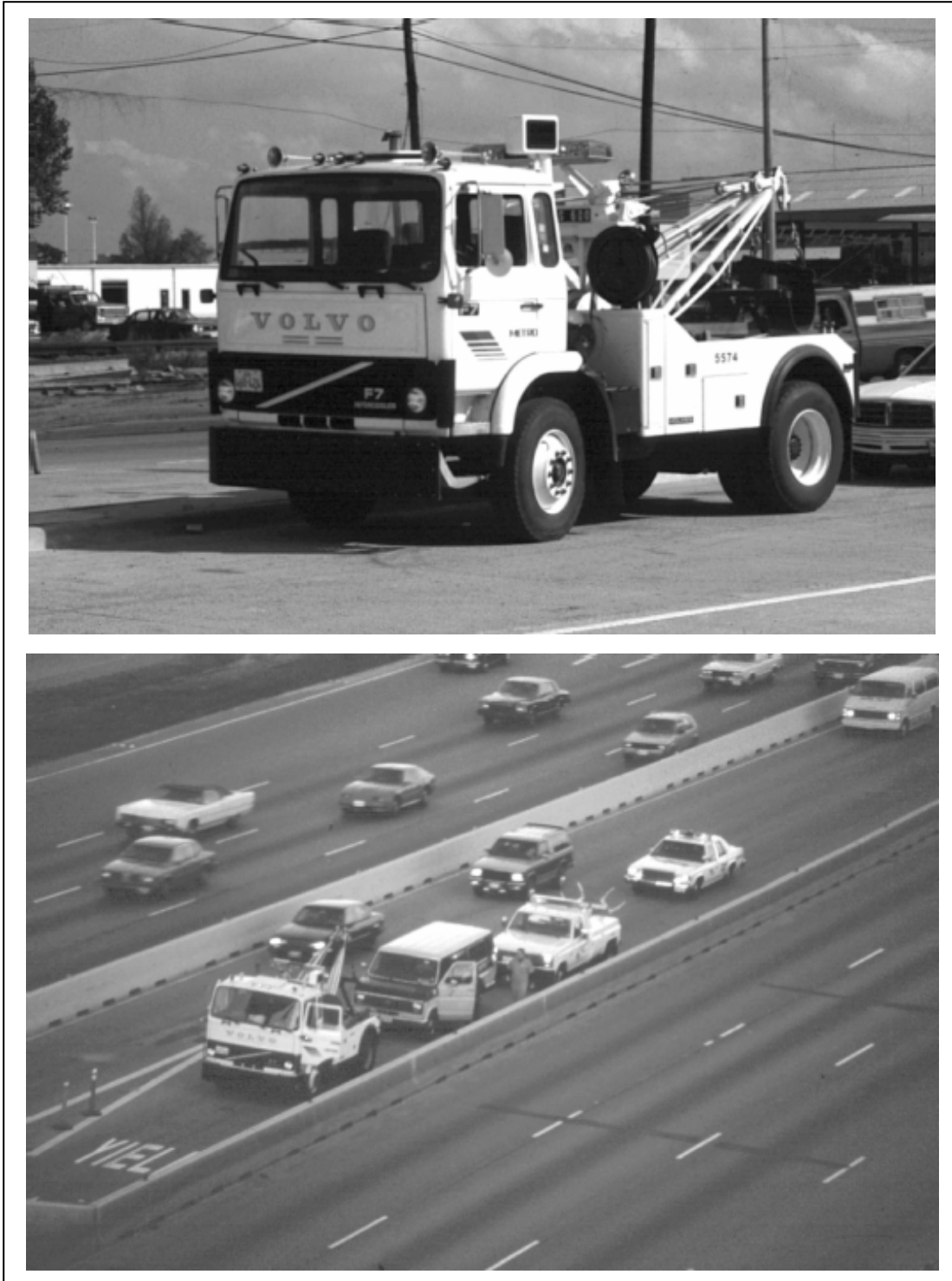
Figure 3-31. METRO Tow Truck and Response to Incident in Houston, Texas. (Short tow truck wheelbase can turn around in 20-foot [6.1 m] lane)
