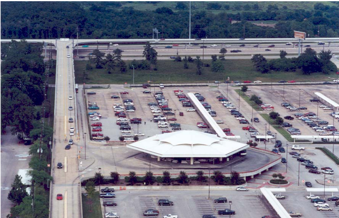
Figure 4-20. Kuykendahl Park-and-Ride Lot Showing Crossover Traffic at Bottom of T-ramp on I-45 (North Freeway) in Houston, Texas.
