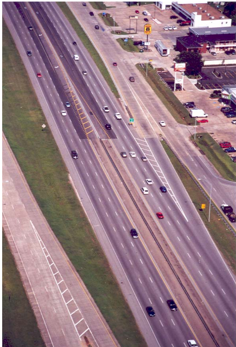
Figure 4-48. Start/End of Concurrent Flow Lanes along I-10 (Katy Freeway) in Houston, Texas.
