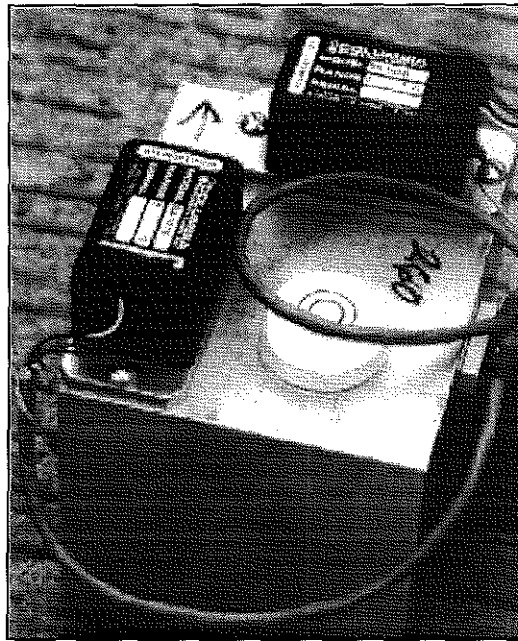
Figure 2.3.1a. Accelerometers in Triaxial Arrangement.
