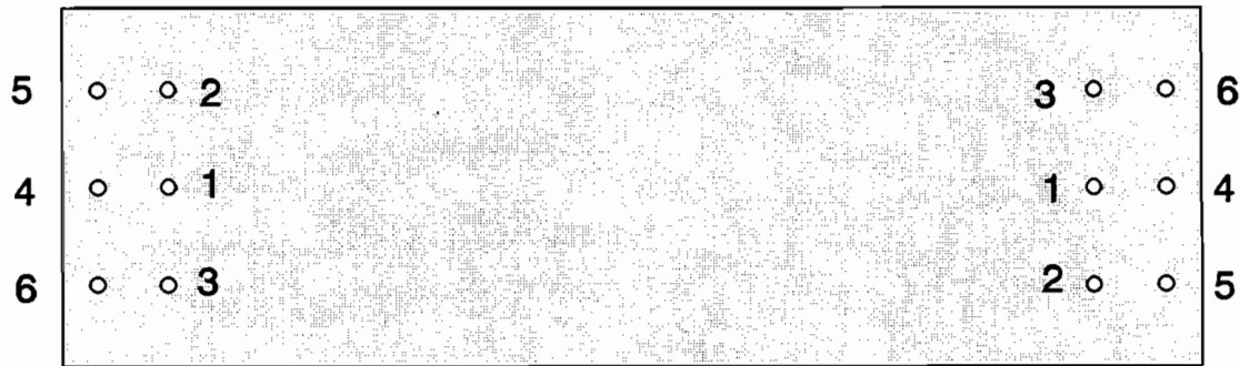
Figure 4.7 Stressing sequence for external vertical post-tensioning bars
