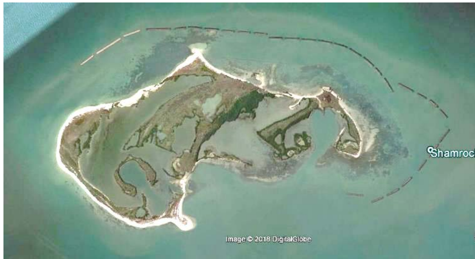
Figure 10. Shamrock Island in 2016 Showing New Set of Shoreline Protection Devices, including Submerged and above Water Rock Breakwaters.
