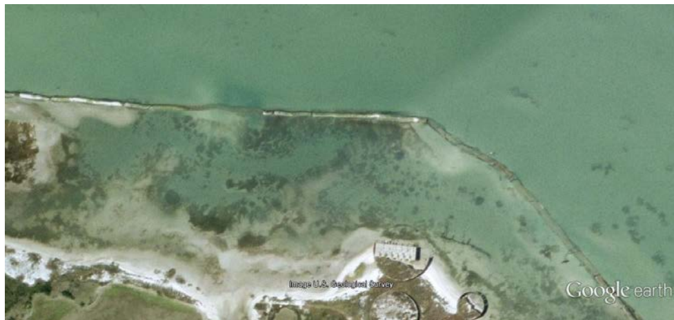
Figure 9. Close-Up of Geotextile Tubes in 2004 Failing.
