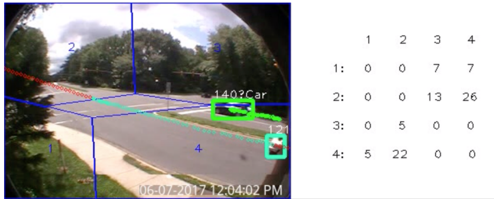
FIGURE 3. Polynomial curve fit on the tracks of 121 (Red extensions at start and end)
