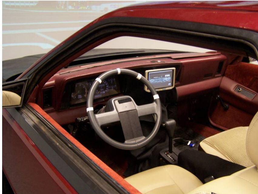
Figure 10. View of the inside of the simulator cab Note: The instrument panel configuration is from a prior study.
