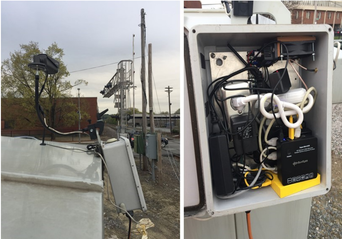
Figure 5. Video Data Capture Equipment at the Brighton St. Crossing
