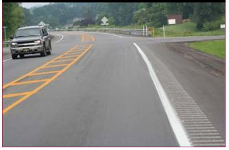
Figure 9. Cross hatching in median at an intersection with left-turn bay.
