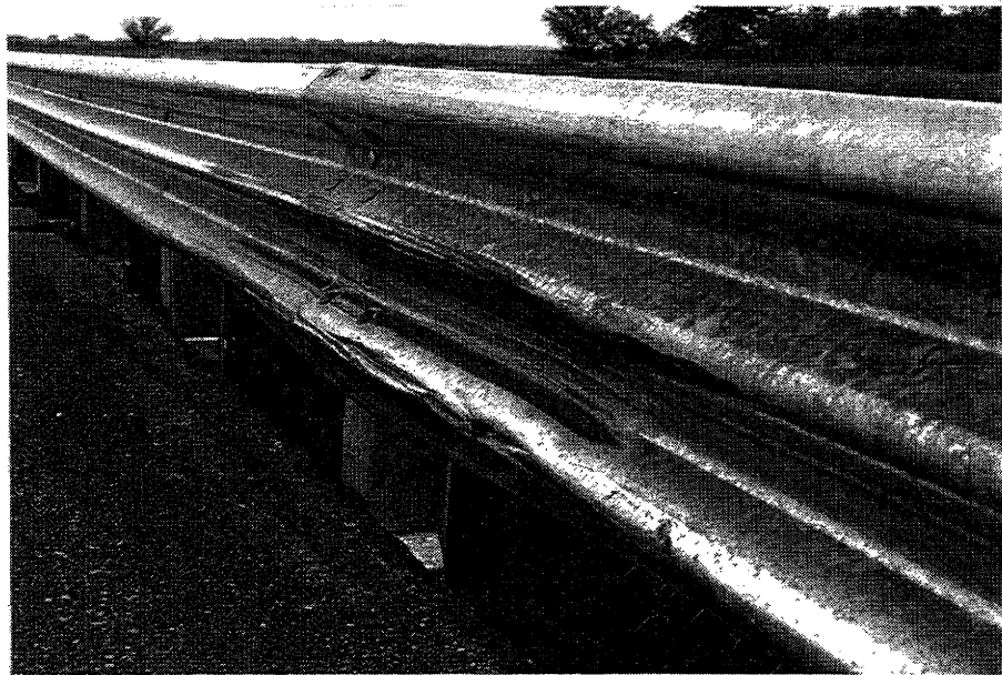
Figure 6. Oregon side-mounted bridge railing after test 7069-17.
