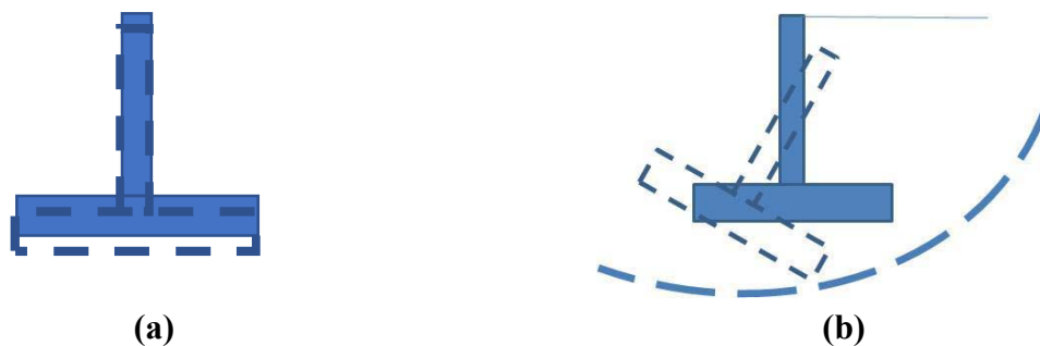
Figure E.1-2. Schematic. Service limit states for spread footings. (a) Settlement, (b) Overall stability.
