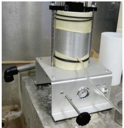
Figure 43. Laboratory flexible-wall asphalt permeameter.
