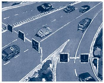
Figure 28. Junction control scheme on German autobahn system.
