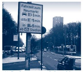
Figure 26. Travel time comparison display on Cologne arterial.
