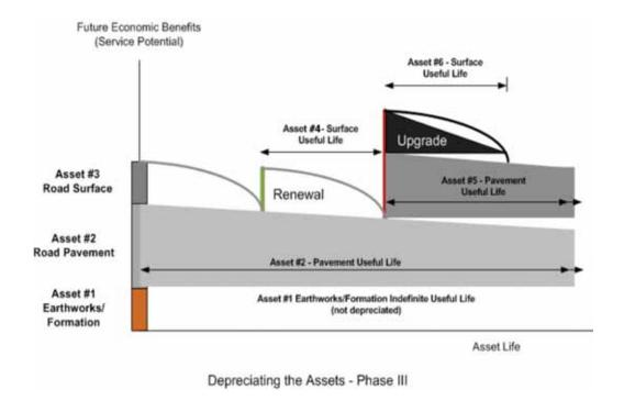
**Figure 6.** Illustration of methods of accounting for pavement assets by component (IPWEA).
