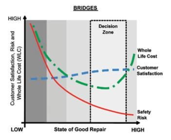
**Figure** 15. Consideration of multiple factors influencing the state of good repair for bridges at Transport for London.
