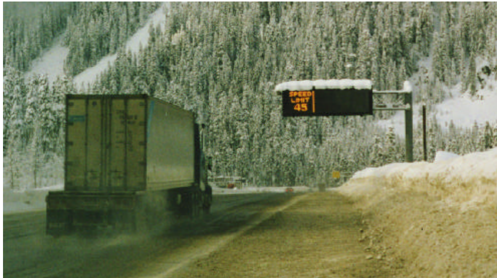
Variable speed limit signs, first observed on a tour of European highway operations, allow speed limits to be adjusted as weather conditions change on Washington State highways.
