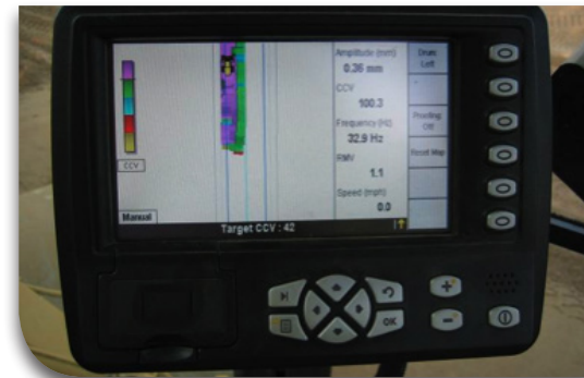
Caterpillar on-board display unit with AcuGrade® software.
