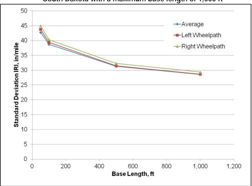
Figure 5.5 Impact of base length on variation in IRI for data collected in South Dakota with a maximum base length of 1,000 ft
