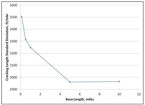
Figure 7.2 Change in variability of cracking length by sample length
