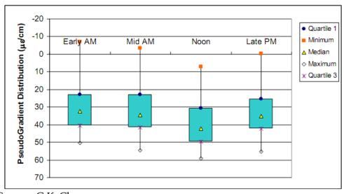
Figure 6.3 Observed temperature gradient in a curled-down segment of jointed concrete (5)
