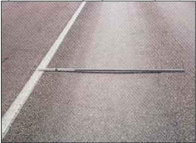
Figure 4.1 Use of straightedge for measuring rut depth
