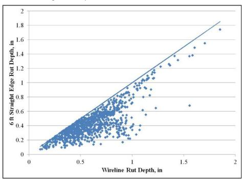
Figure 4.8 Comparison of 6-foot straightedge and wireline rut depths in the right wheelpath
