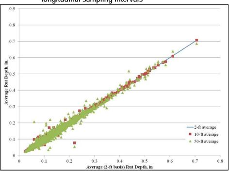
Figure 4.5 Average rut depth based on 2-foot, 10-foot, and 50-foot longitudinal sampling intervals
