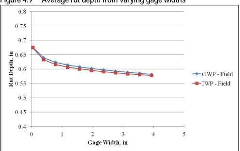
Figure 4.9 Average rut depth from varying gage widths
