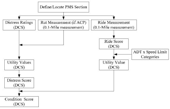
Figure 6. Flowchart. TXDOT Process Used to Calculate PMIS Condition Score (Wu et al., 2010)
