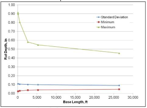
Figure 4.10 Impact of base length on standard deviation, minimum, and maximum rut depth
