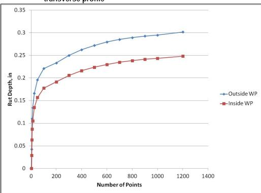
Figure 4.3 Average rut depth based on varying number of points within the transverse profile
