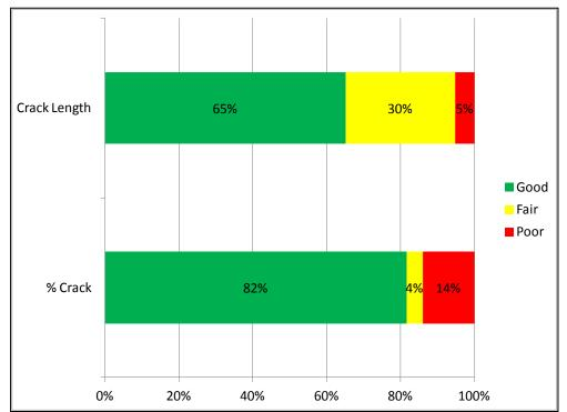
Figure 7.3 Condition of pilot study corridor in terms of cracking using a 0.1mile base length
