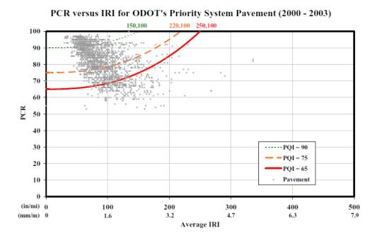
Figure 26. Graph. Linear PCR with Power IRI function for priority System (Reza et al., 2005)
