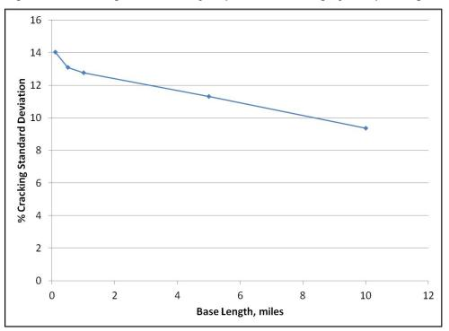
Figure 7.1 Change in variability of percent cracking by sample length
