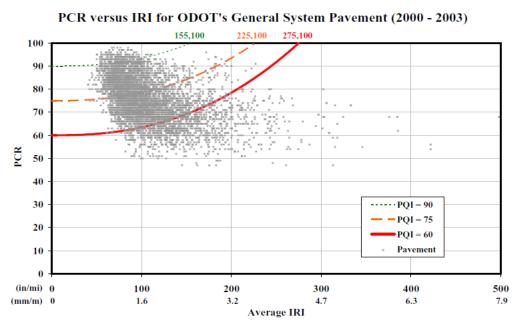
Figure 27. Graph. Linear PCR with Power IRI function for General System (Reza et al., 2005)
