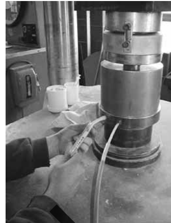
Pore water is extracted from a mortar sample as part of CPTP's research into incompatible concrete materials.
