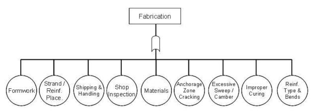
Figure 3-9 Portion of the precast concrete girder bridge fault tree showing the Fabrication Category only, with several Basic Events provided.
