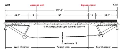
**Figure 3-4** Sketch showing the elevation of de la Concorde overpass; the simple central span of the bridge consisted of adjacent box girders, which rested on a beam seat that was built into the thickened slab that cantilevered from the abutments at each end (taken from [52]).
