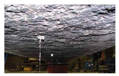
**Figure 3-5** Photo of the bottom face of a tested beam subjected to fire while in service showing that the concrete has deteriorated such that sufficient pathways through the concrete to the bottom layer of prestressing strands have developed (taken from [56]).
