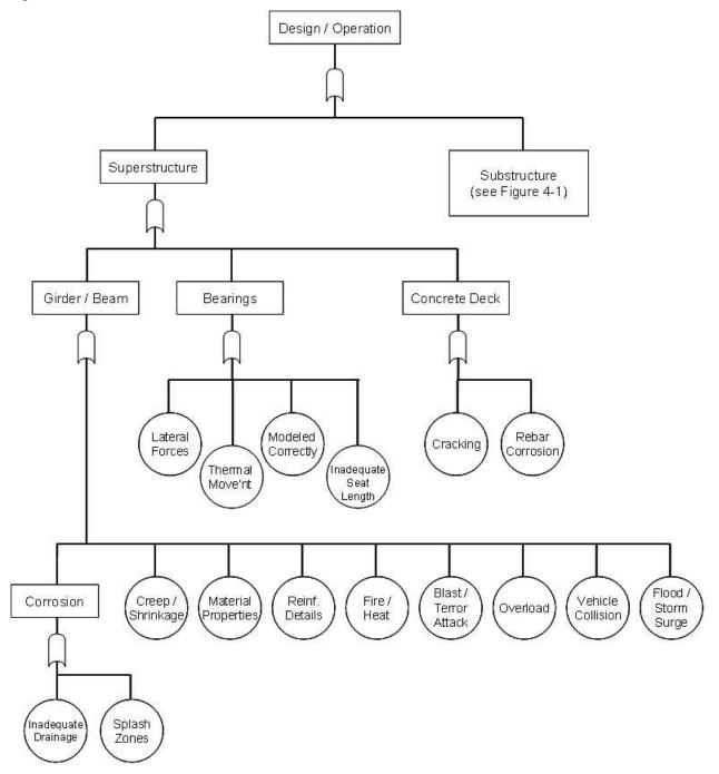
**Figure 3-2** Portion of the precast concrete girder bridge fault tree showing the Design and/or Operation category for superstructures only, with several Events and Basic Events provided.
