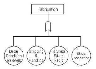
**Figure 2-12** Portion of the steel girder bridge fault tree showing the Fabrication Category only, with four Basic Events provided.
