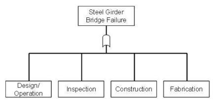
Figure 2-1 Steel girder bridge fault tree, showing top categories only which include Design and/or Operation, Inspection, Construction, and Fabrication.
