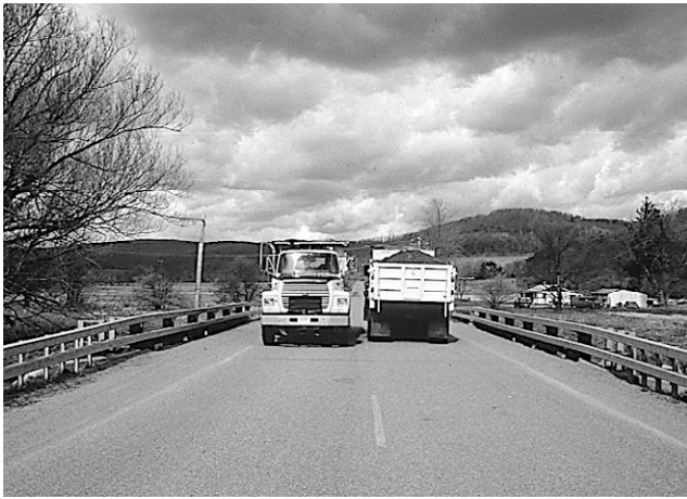
Figure 14—Load testing of trucks in load position 3. Note the location and direction of each truck.
