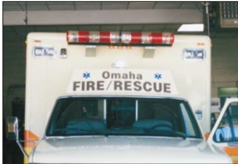
Rescue vehicle equipped with signal pre-emption strobe
