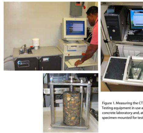
Figure 1. Measuring the CTE of concrete. Testing equipment in use at the FHWA concrete laboratory and, at left, a concrete specimen mounted for testing.
