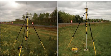
Figure 192. A Trimble GPS base station (left) and a TopCon GPS base station (ICPF WisDOT demo).
