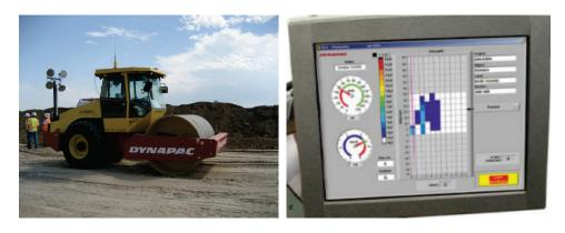
Figure 19. A single-drum Dynapac roller equipped with roller-integrated CMV measurement system and on-board display unit with DCA  $^{\tiny (\!R\!)}$  software.
