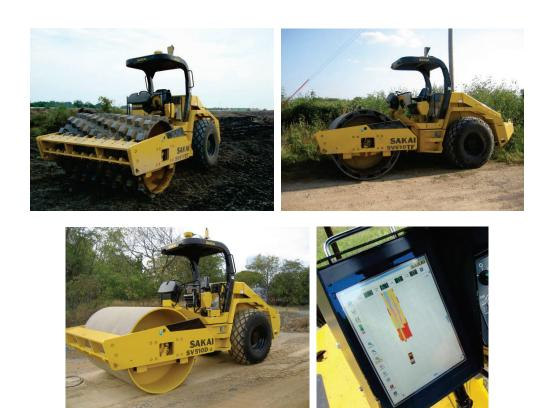
Figure 20. Sakai rollers (padfoot and smooth drum) equipped with roller-integrated CCV measurement system and on-board display unit with Aithon- $MT^{@}$  software.
