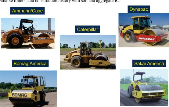
Figure 7. Single smooth drum IC rollers.
