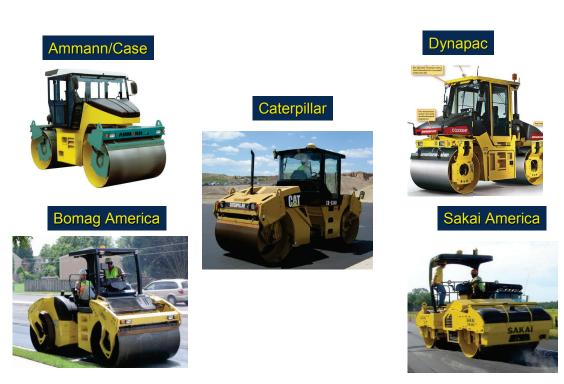
Figure 8. Double drum IC rollers.
