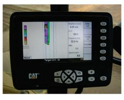
Figure 18. Caterpillar rollers (padfoot and smooth drum) equipped with roller-integrated MDP and CMV measurement systems on-board display unit with AcuGrade® software.
