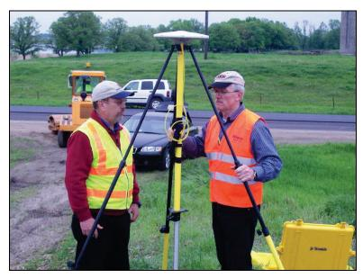
Figure 13. A Trimble GPS base station (ICPF MnDOT demo).
