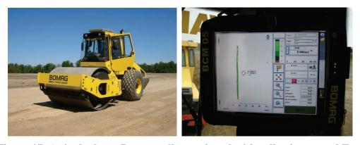
Figure 17. A single-drum Bomag roller equipped with roller-integrated  $E_{VIB}$  measurement system on-board display units with BCM-05  $^{\!@}$  software.
