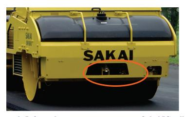
Figure 6. Infra-red temperature sensor on a Sakai IC roller.
