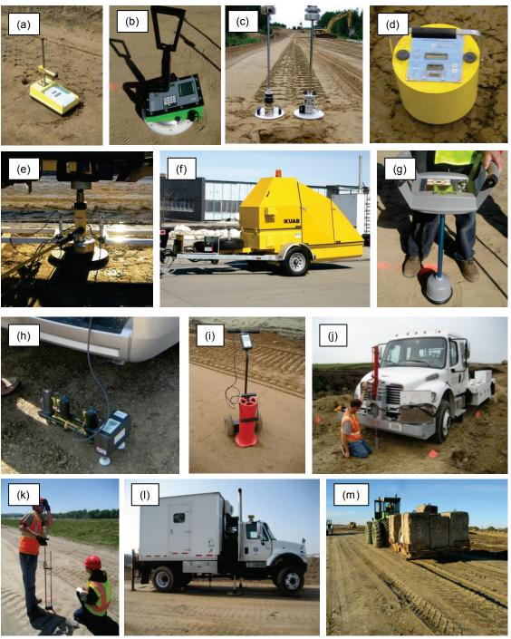
Figure 28. Various in-situ QC/QA test measurements: (a) nuclear moisture-density gauge; (b) electrical density gauge; (c) light weight deflectometers; (d) soil stiffness gauge; (e) static plate load test; (f) falling weight deflectometer; (g) Briaud compaction device; (h) seismic pavement analyzer; (i) Clegg hammer; (j) shelby tube sampling; (k) dynamic cone penetrometer; (l) static cone penetrometer; and (m) heavy test rolling.
