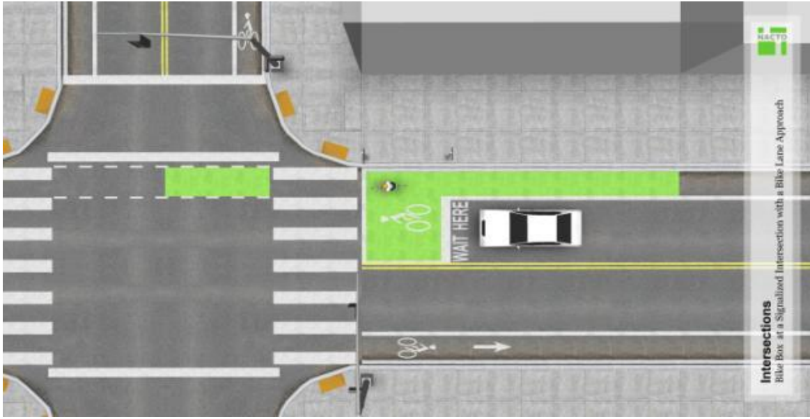
Figure 1. Illustration of a Typical Bike Box. Image from Urban Bikeway Design Guide, Second Edition , by NACTO. Copyright © 2014 National Association of City Transportation Officials. Reproduced by permission of Island Press, Washington, D.C.
