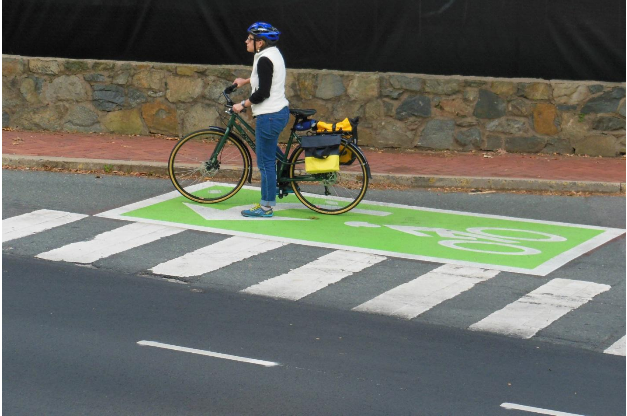
Figure 2. Photograph of a Bicyclist in a Two-Stage Left-Turn Box
