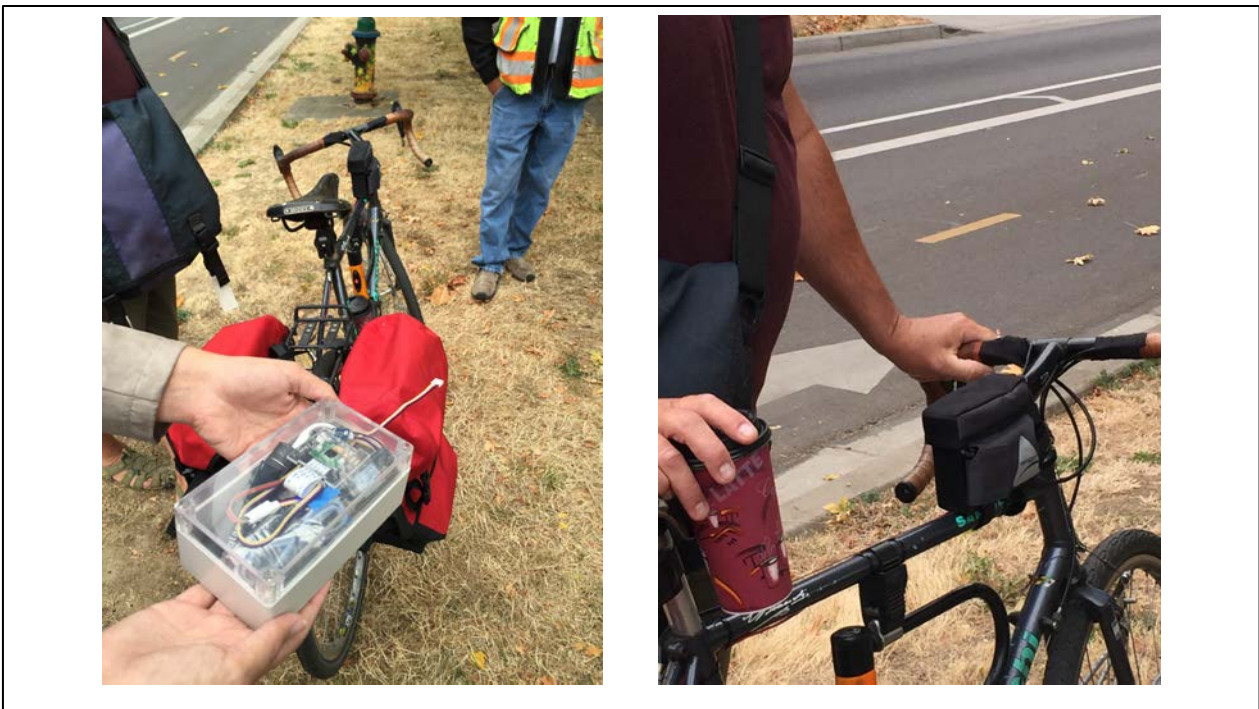
Figure 7: Prototype Bike Computer in a box and stuffed into small bike bag.
