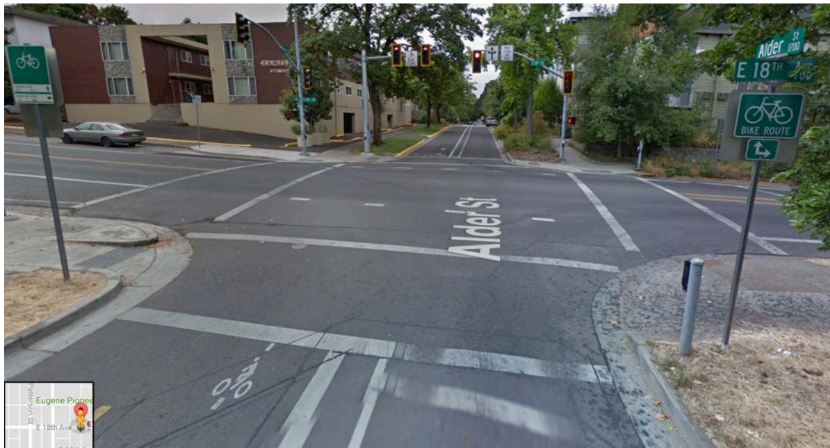
Figure 3: Intersection of Alder and 18th (looking south). Intersection of Alder and 18th (looking south) with signal phases for bike only (left) and car only (right) and the terminal loop detector bottom left (many people on bike wait in the crosswalk not knowing what the bike loop detector symbol is for). (Source: Google Street View, August 2017 (accessed 7/4/2018)).
