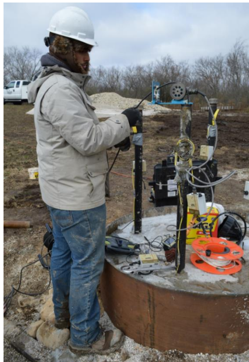
Figure 41: TIP testing via the probe method utilizes a depth encoder pulley that logs the probe depth as it is raised from the bottom of the access tube.
