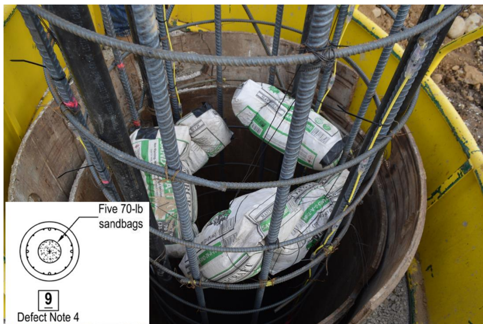
Figure 27: Defect 9 consisted of five 70 lb sandbags placed inside the reinforcing cage for Test Shaft 2 at a depth of 12 ft. Defects 6, 7, and 8 are presented in the next section.
