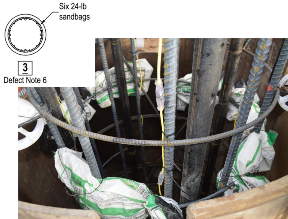
Figure 24: Defect 3 consisted of six 24 lb sandbags tied concentrically around the edge of the reinforcing cage for Test Shaft 1 at a depth of 21 ft.
