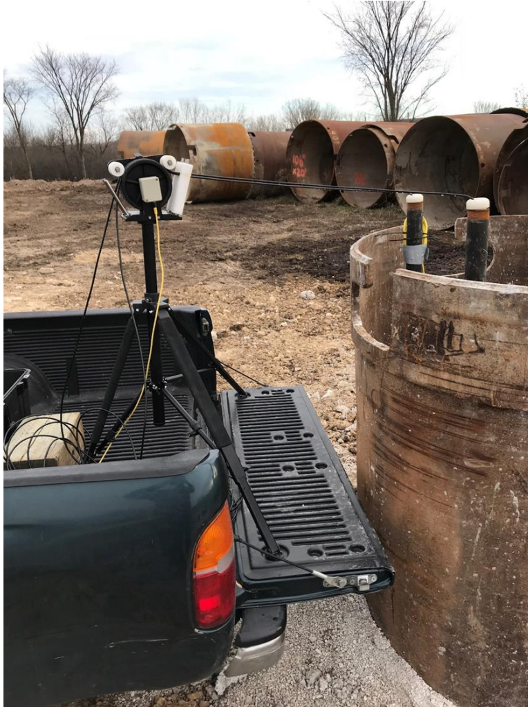
Figure 44: CSL testing utilized equipment by Olson Instruments, Inc., including a dual depth encoder pulley used to lower the source and receiver probes down two access tubes simultaneously.
