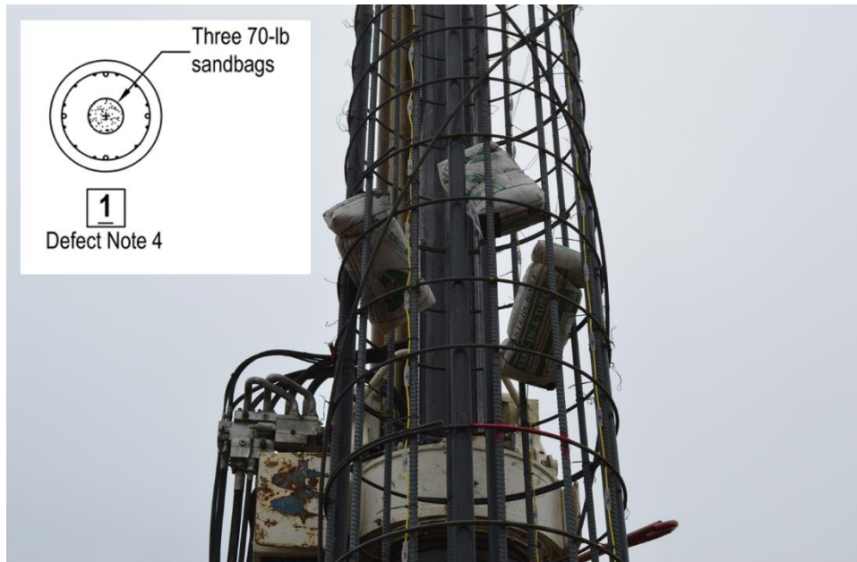
Figure 22: Defect 1 consisted of three 70 lb sandbags tied inside the reinforcing cage for the Control Shaft.
