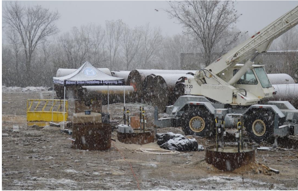
Figure 42: TIP testing by probe method for Test Shaft 2 was completed with ambient temperatures near 30° F.
