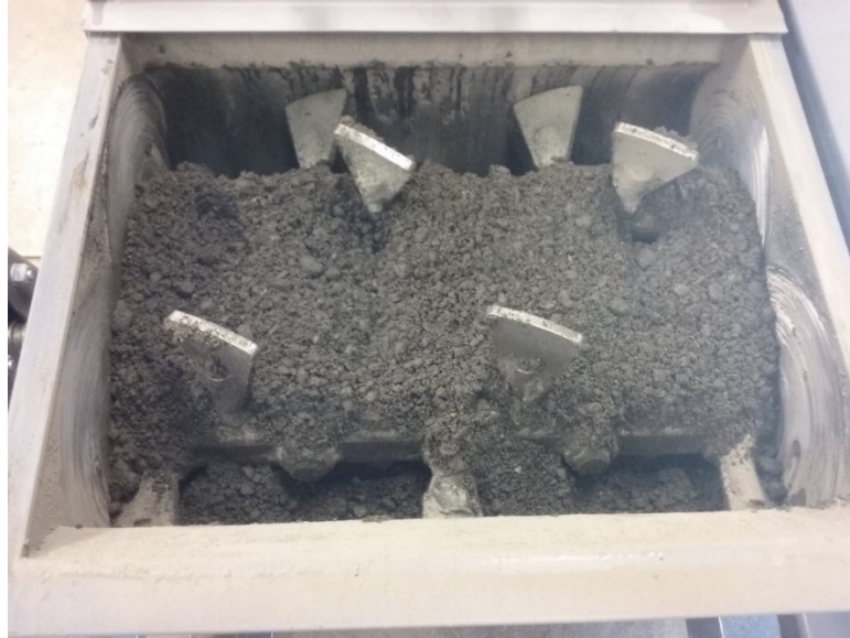
Figure 3-3 RAP after Mixing with Cement, Water, and Foamed Asphalt Cement
