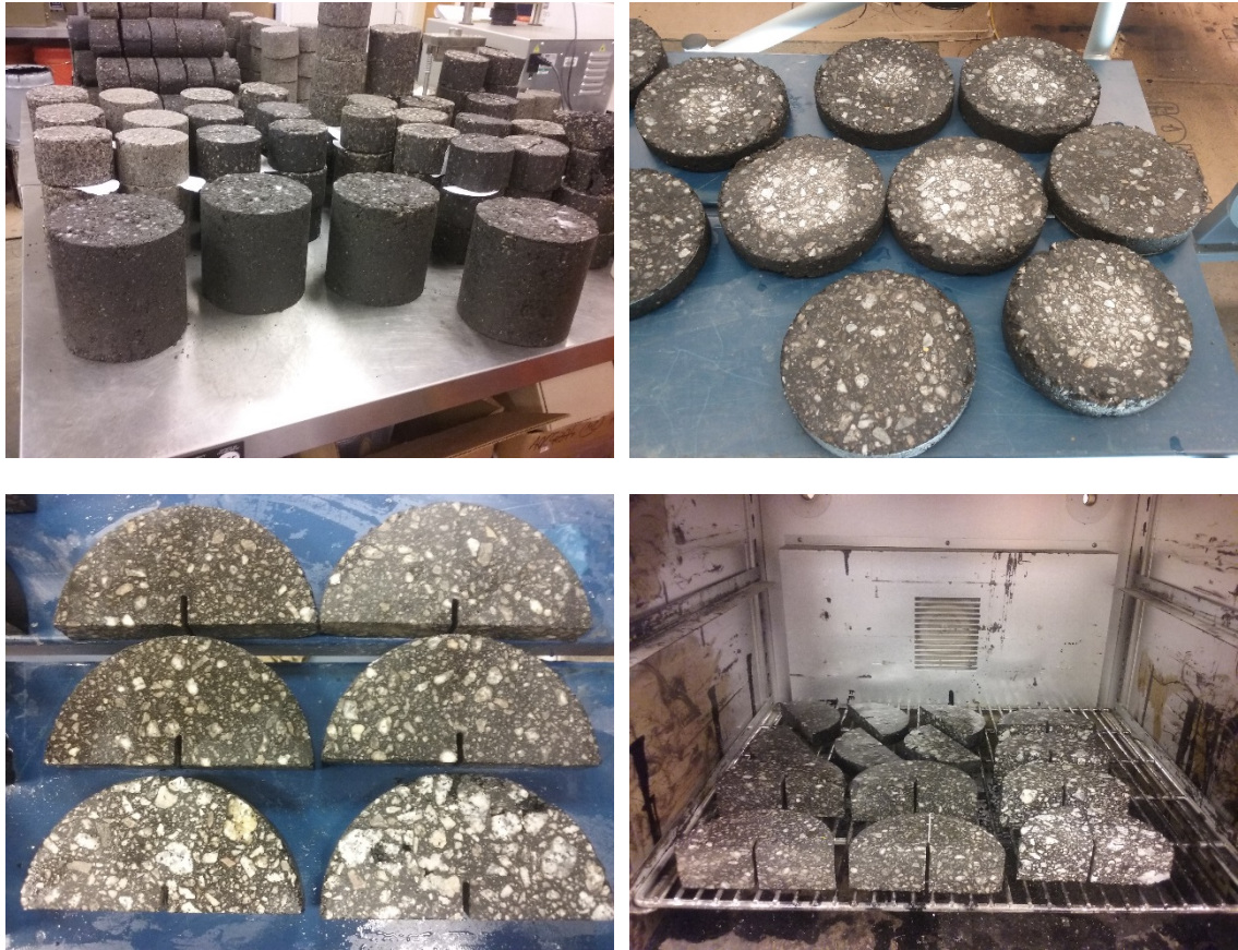
Figure 2-9 Specimen Preparation for Semi Circular Bending Test
