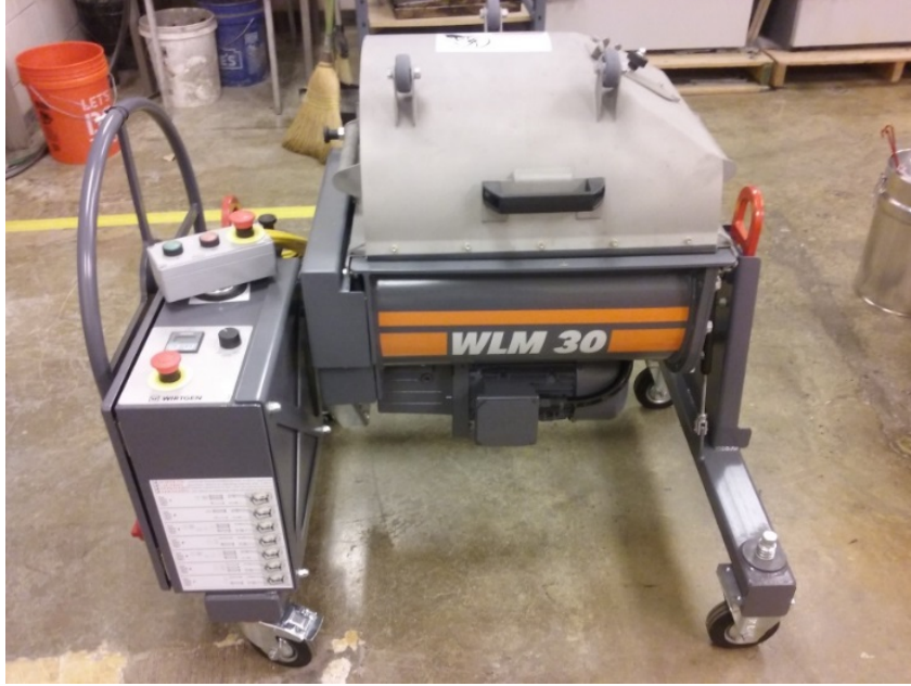
Figure 3-1 Foamed Asphalt Mixer (Wirtgen Model: WLM 30)
