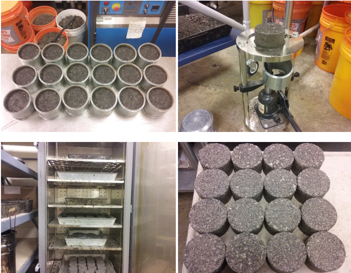
Figure 3-5 Specimen Extrusion and Oven Curing
