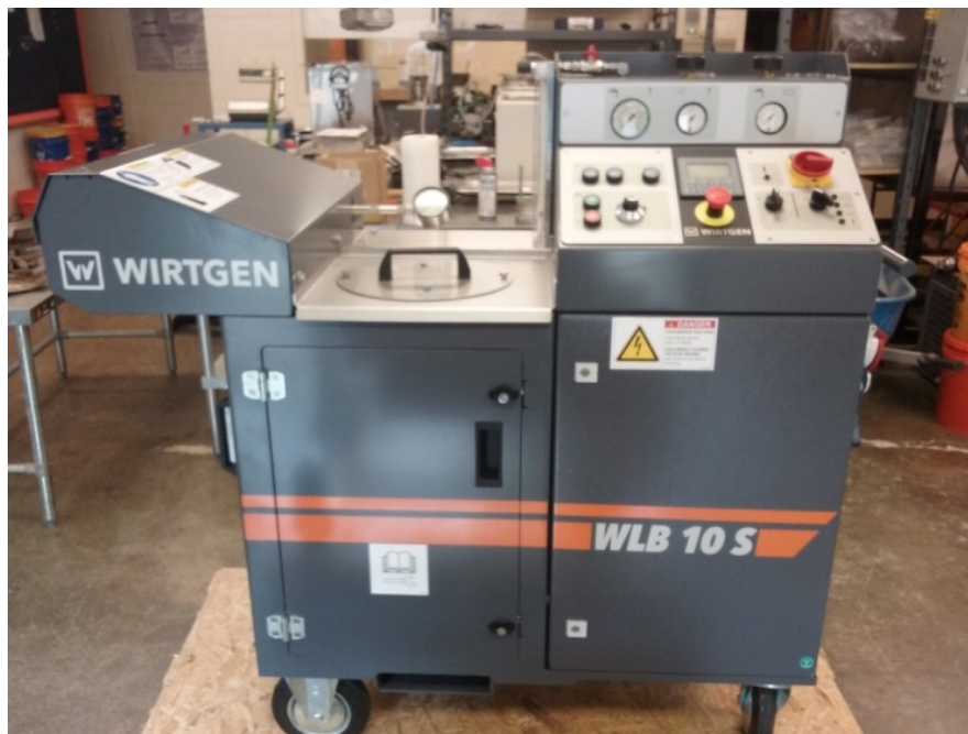
Figure 2-5 Wirtgen Asphalt Cement Foaming Equipment (Model: WLS 10S)
