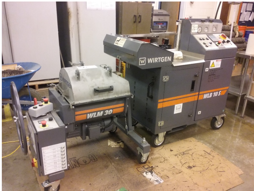
Figure 3-2 Laboratory Scale Foamed Asphalt Plant
