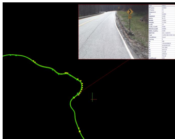
Figure 4-7 An example of a detected traffic sign (W1-8) on the State Route 2
