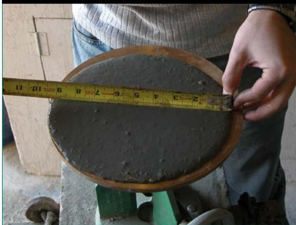
Figure 5. ASTM C1437 flow test on UHPC. (6)
