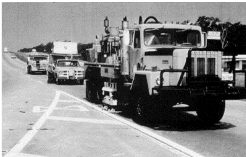
Figure 9.3 Photograph of RDD Testing on IH-10 near Orange, Texas
