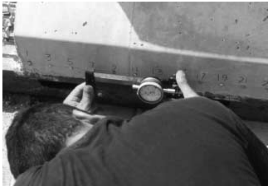
Figure 5.3: Performing a Measurement with DEMEC Gauge
