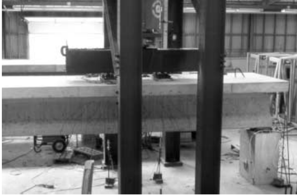
Figure 7.2: Load Application Components—Test H0R-D-66
