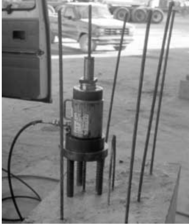
Figure 4.5: Pull-out Test in Progress
