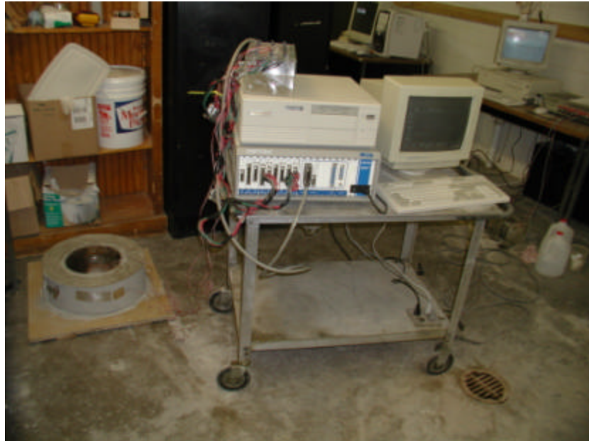
Fig. III-1 The data acquisition system used for monitoring the strains on the inner surface of the steel ring and on the outer surface of concrete.
