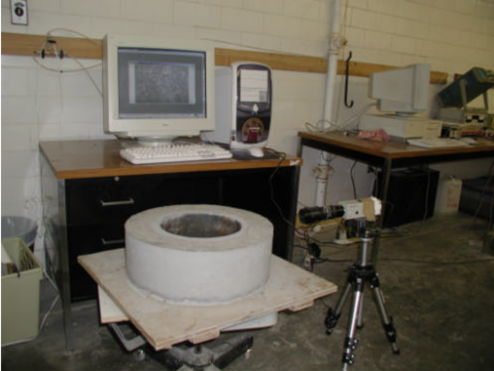
Fig. II-1. The experimental setup monitoring surface cracking on the concrete ring.
