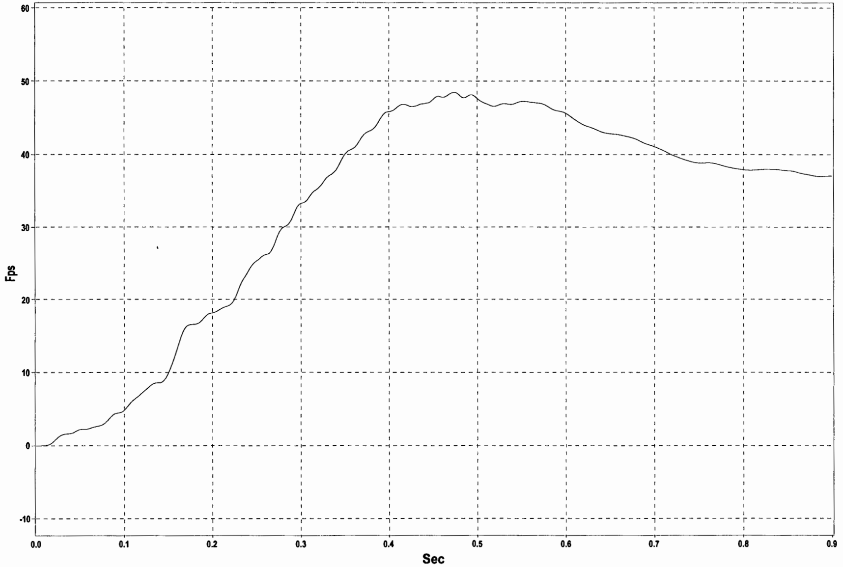
W6: Lateral Occupant Impact Velocity - Test OLS-3 (EDR-4)
