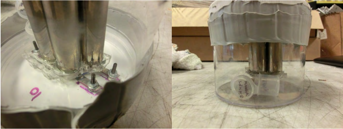
Figure 15 - An electrolyte exposure chamber containing four 18650 cells after 20 days of exposure. Cloudiness can be seen on the cell walls due to the electrolyte vapor.
