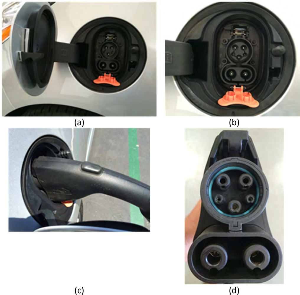
Figure 20 - Visual inspection of a) the vehicle charge receptacle, b) the vehicle charge receptacle (close-up), c) the charger coupler, and d) the charger coupler (close-up).
