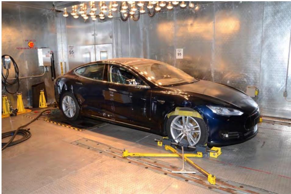
Figure 30 - The test vehicle installed on the dynamometer. Solar load lights are used to provide illumination for the image, but were not used during testing. The coiled Level 3 charge cable can be seen on the left.
