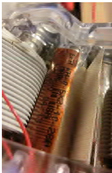
Figure 61 - Thin film heater attached to cell.
