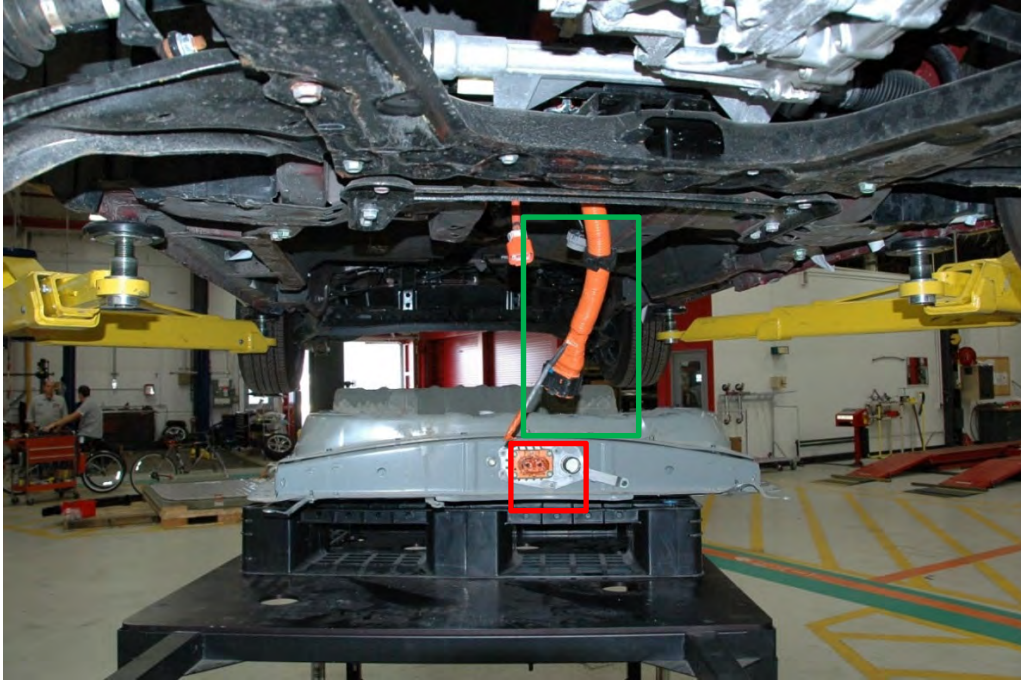
Figure 18 - Manufacturer C vehicle; RESS high voltage connection. The high voltage cable from the vehicle (green box) connects directly to the RESS (red box). The RESS was removed from the vehicle for demonstrative purposes. The high voltage connection can be accessed without RESS removal.
