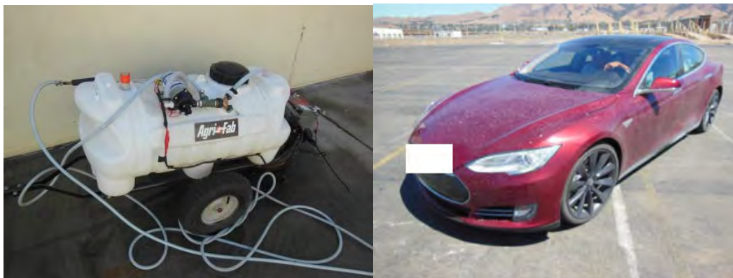
Figure 24 - Salt spray applicator (left) and an example of a vehicle after salt spray application (right).
