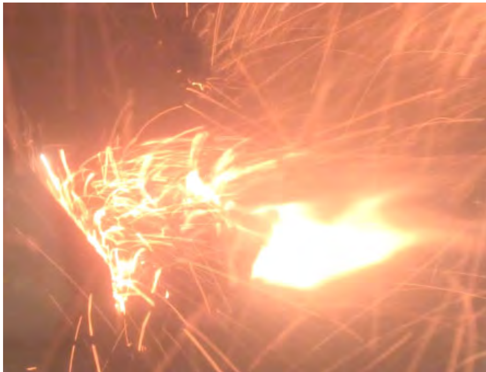
Figure 30 - Cylindrical cell undergoing thermal runaway; off-the-shelf heater method.
