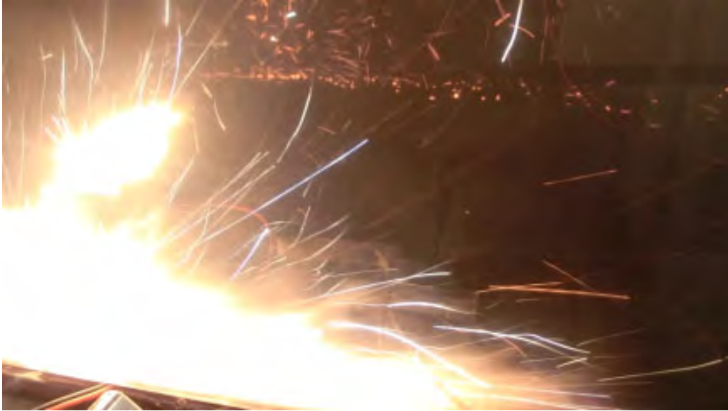
Figure 15 - Cylindrical cell undergoing thermal runaway; nichrome wrap heater method.
