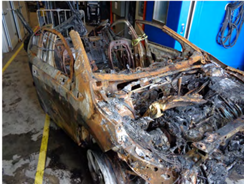
Figure 214 -GM Volt PHEV post fire and salt water discharge.
