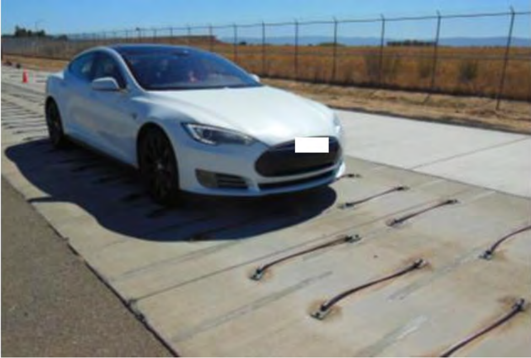
Figure 21 - An example of a vehicle on a rope road (i.e., rough road element).
