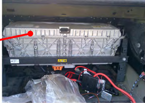
Figure 3 - Example HV RESS external case voltage sensing.
