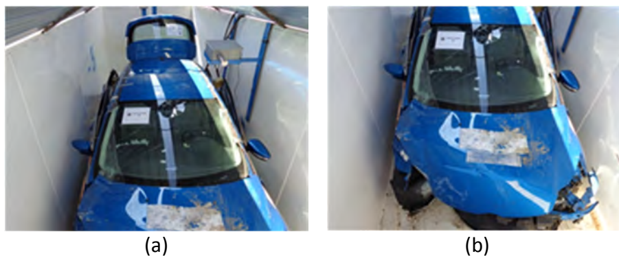
Figure 170 - Ford Focus LP EV setup: a) video camera, and b) the vehicle in its immersion container.
