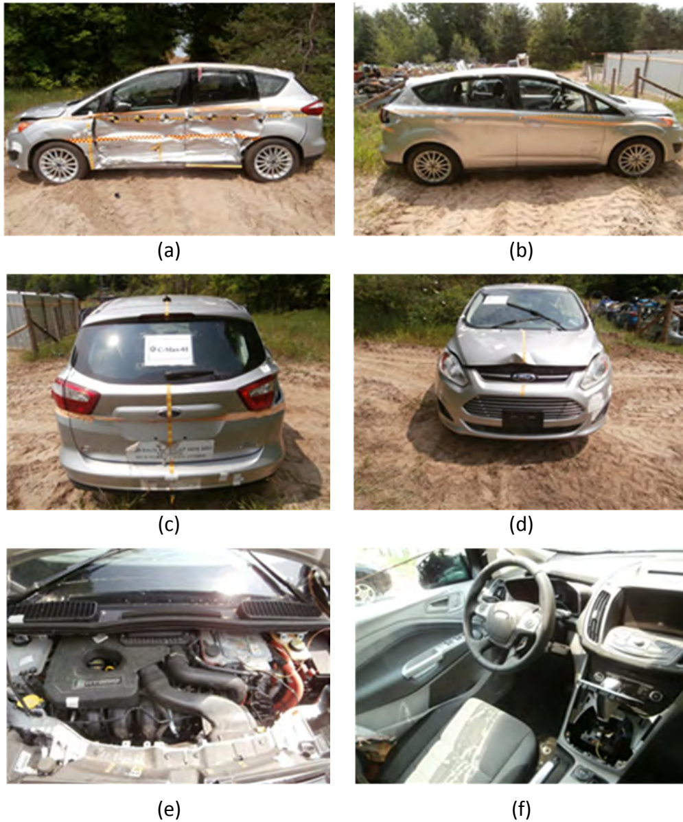
Figure 29 - Ford C-Max HEV post-test vehicle condition: a) left view, b) right view, c) rear view, d) front view, e) engine bay, and f) driver's seat.
