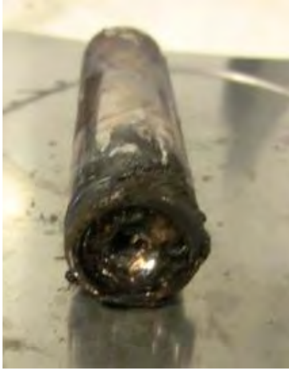
Figure 21 - Cylindrical cell after successful nail penetration trial.
