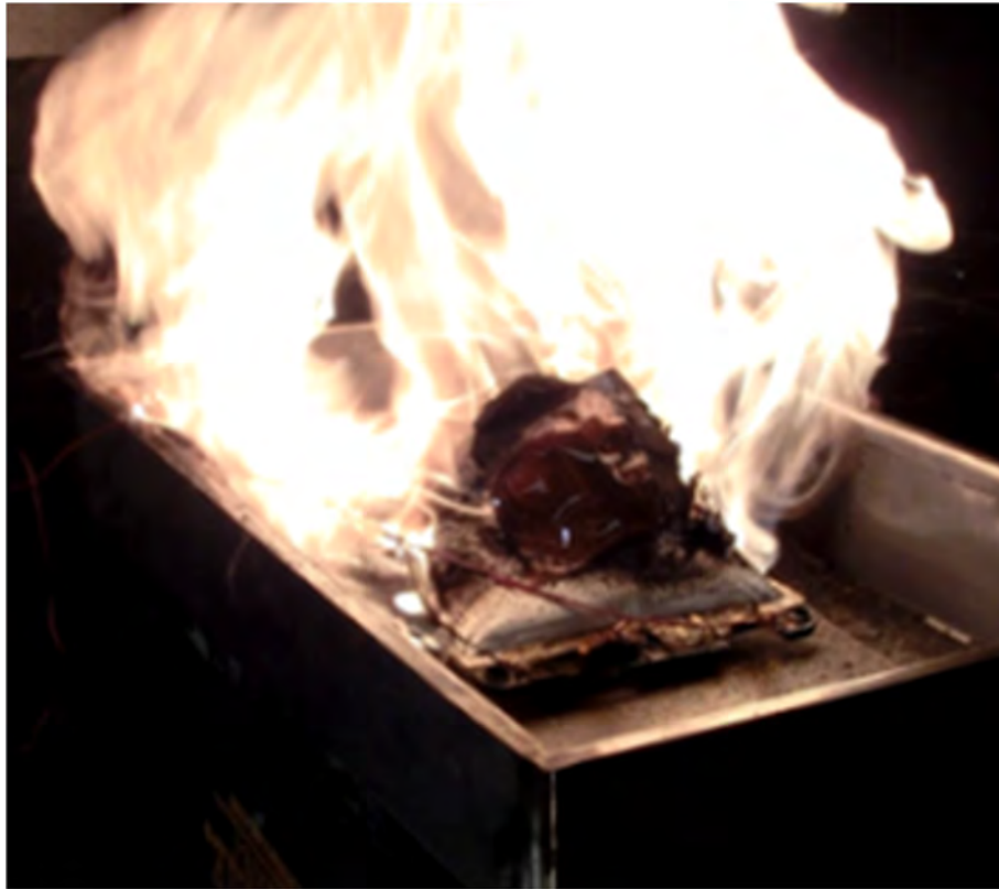
Figure 51 - Ignition of thermal runaway gases from pouch cell.
