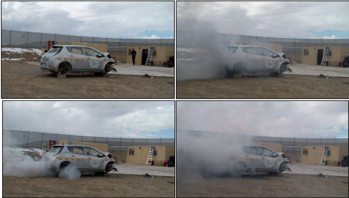
Figure 103 - Top left: 7:07, beginning of first runaway. Top right: 8:16, fourth cell runaway in the first module. Bottom left: 14:47, second module begins after lull. Bottom right: 22:10, several modules into event, ignition coming soon. Between runaways, the smoke cleared and resembled the top left image.
