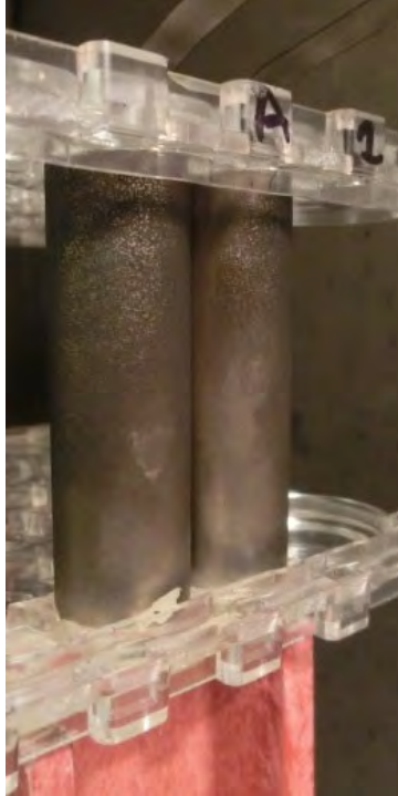
Figure 9 - Cylindrical cell coupon (two cells) after exposure to smoke from smoldering electrical wiring.
