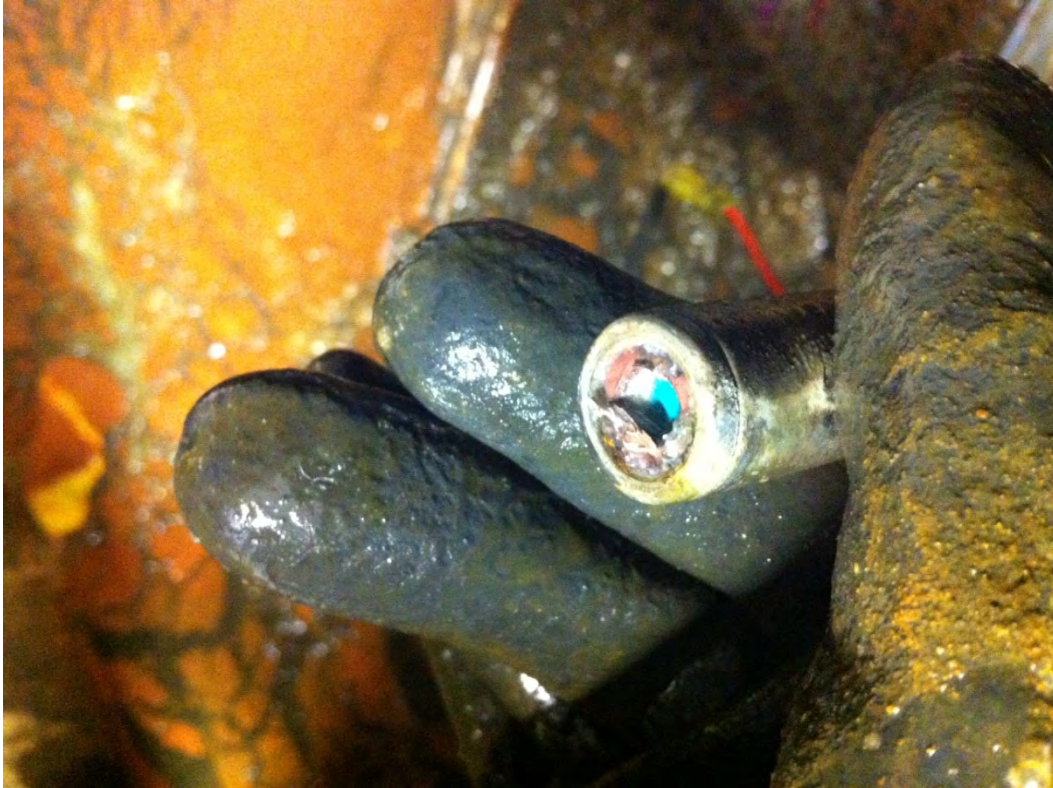
Figure 10 - An example of an 18650 cylindrical cell after a salt bath destructive discharge. The positive terminal has been removed by corrosion, thus exposing the cell interior.
