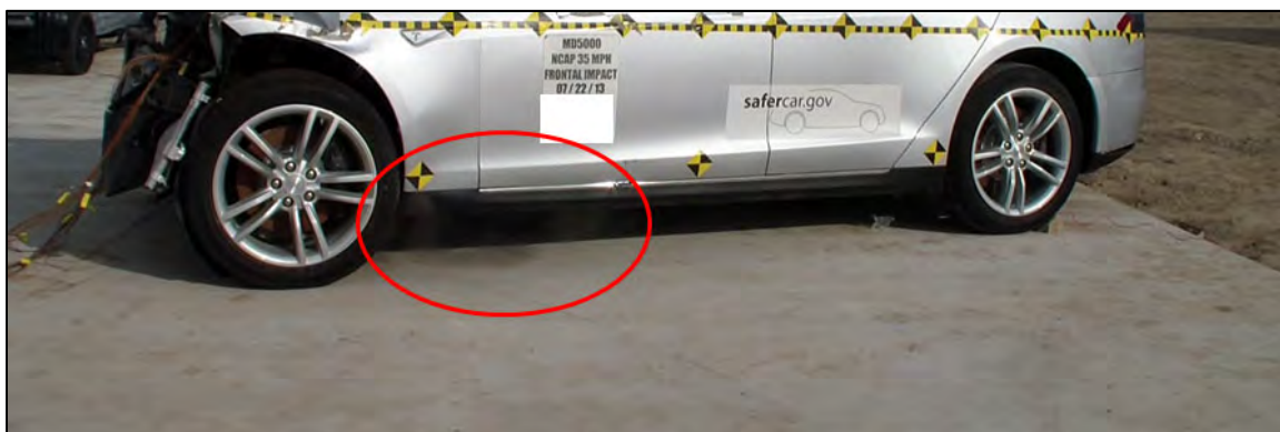
Figure 82 - Smoke escaping the battery pack as a result of thermal runaway of the initiating cell.
