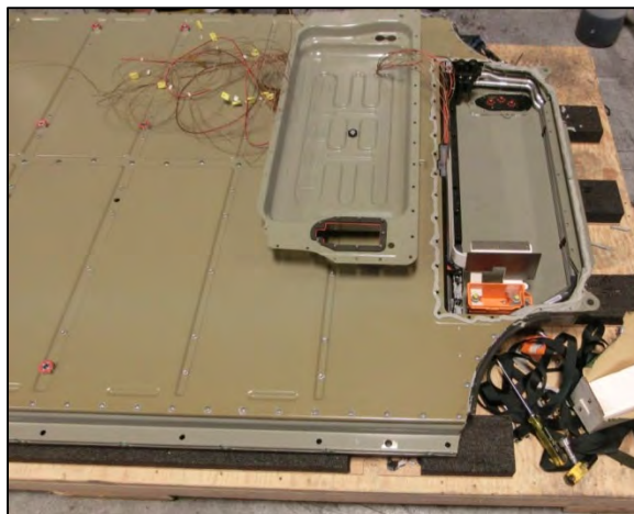
Figure 78 - The cylindrical battery pack with sealant applied to seal the flat main cover to the front cover.
