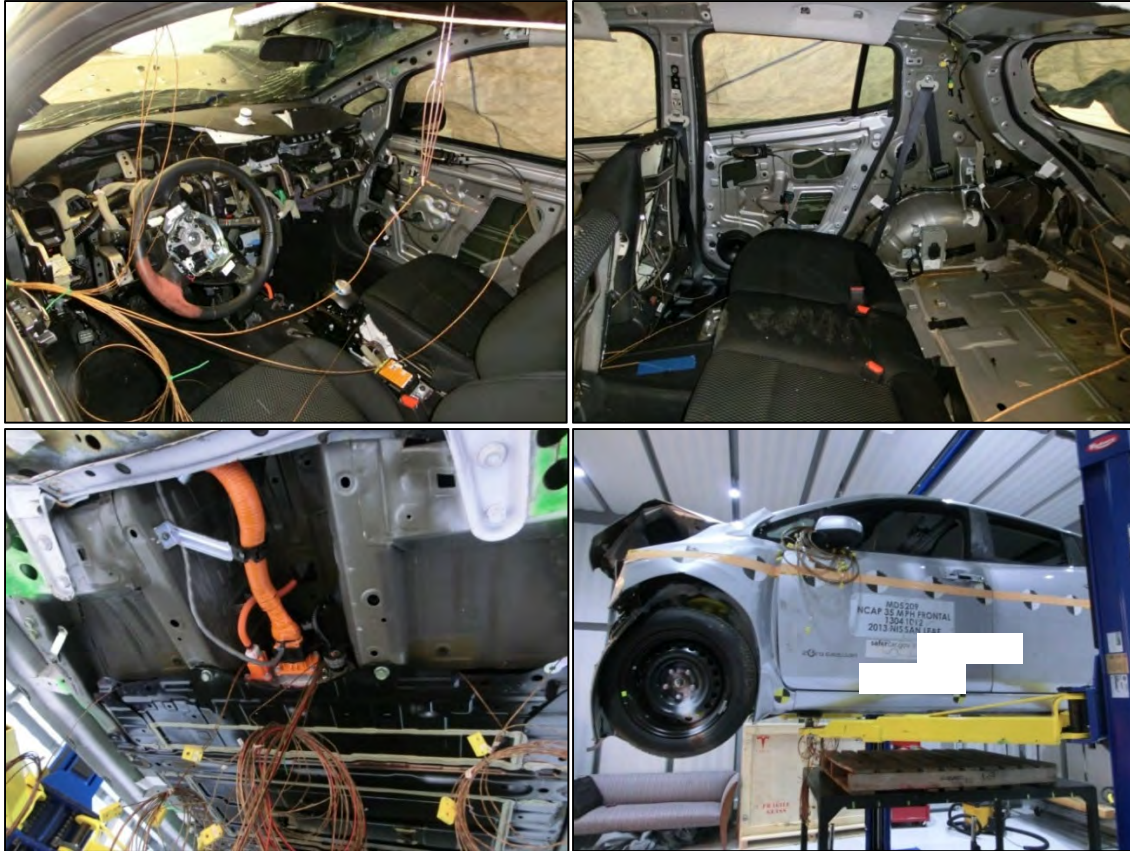
Figure 102 - The Manufacturer C vehicle with thermocouples installed and many flammable materials removed.
