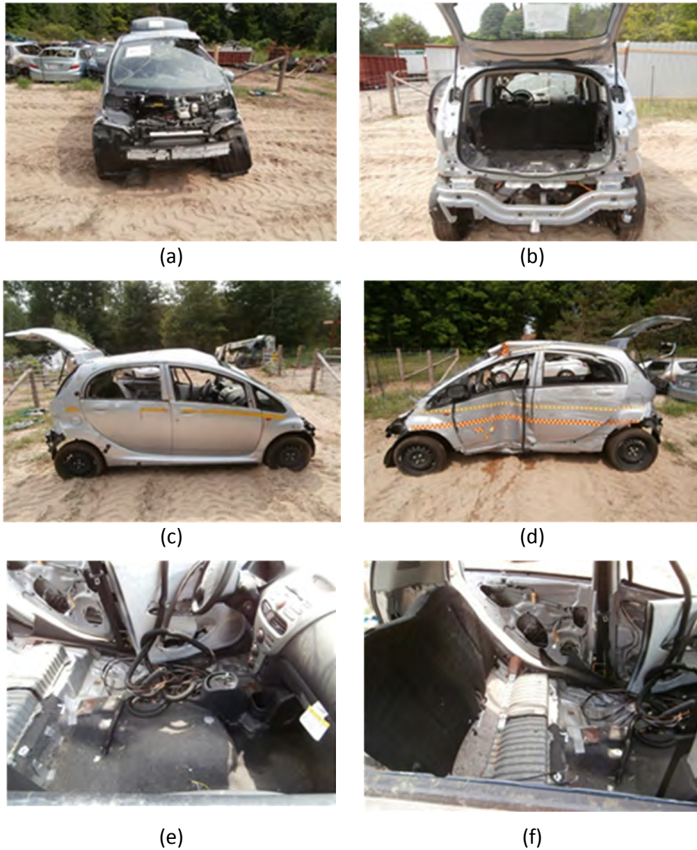
Figure 151 - Mitsubishi iMiev EV post-test vehicle condition: a) front view, b) rear view, c) passenger side view, d) driver's side, e) interior cabin (front), and f) interior cabin (rear).
