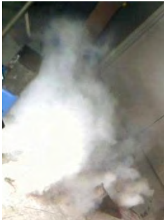
Figure 44 - Prismatic cell undergoing thermal runaway; large film heater Trial #2.
