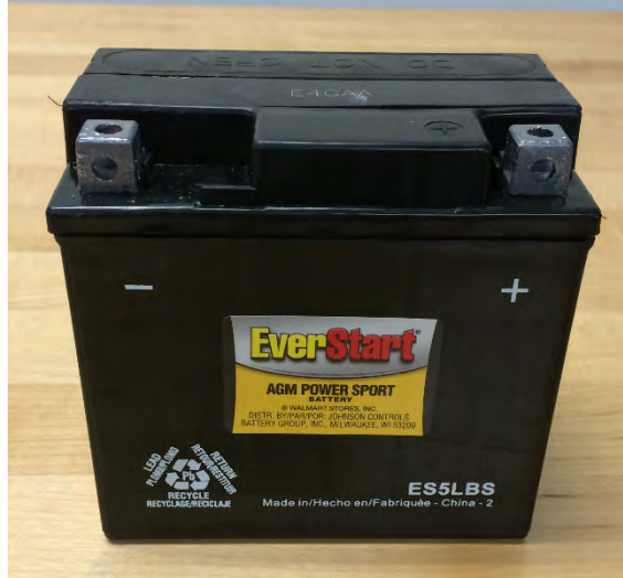
Figure 19 - 12 V lead acid battery.
