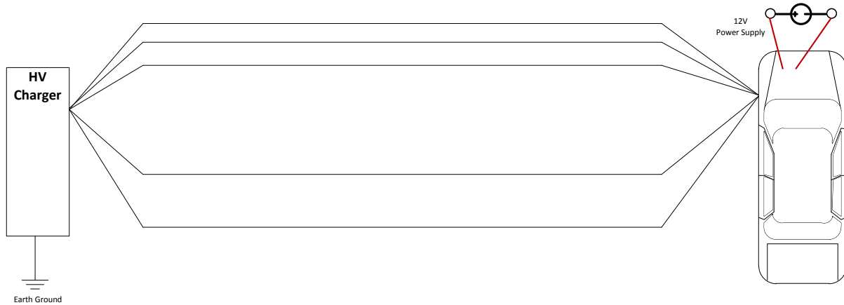
Figure 9 - 12 V Power Supply Connection.
