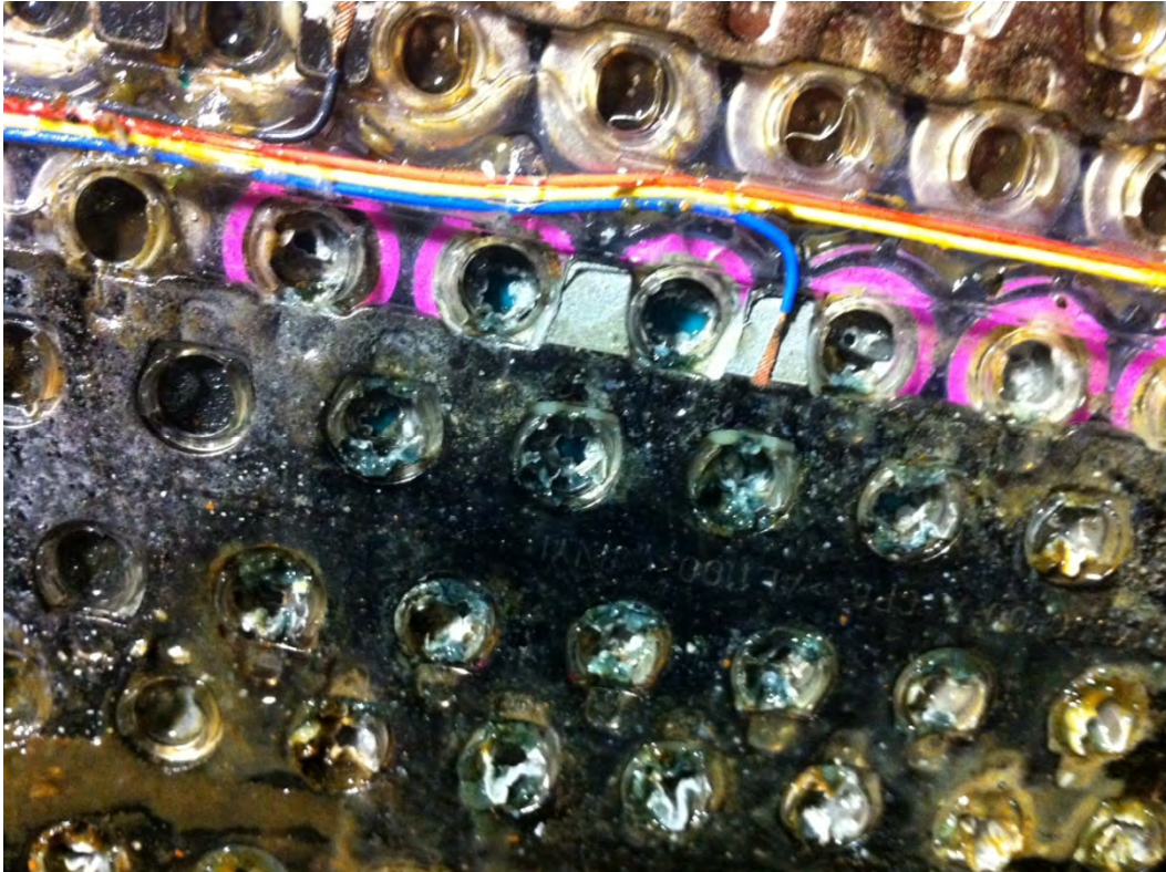
Figure 43 - An example of a Manufacturer A module after a salt bath destructive discharge.
