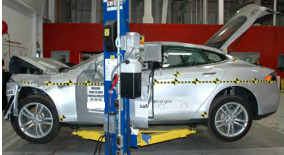
Figure 79 - The frontal crash Manufacturer A vehicle used for the demonstration of SCTRl testing.
