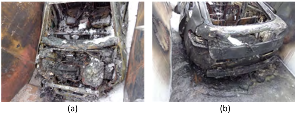
Figure 80 - GM Volt-1 PHEV post-test vehicle condition: a) front view and b) rear view.
