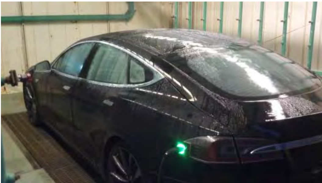
Figure 28 - An example of a vehicle subjected to drizzle chamber charging. Drizzle is simulated by applying a total water flow rate of 12 GPM from the top of the chamber only.
