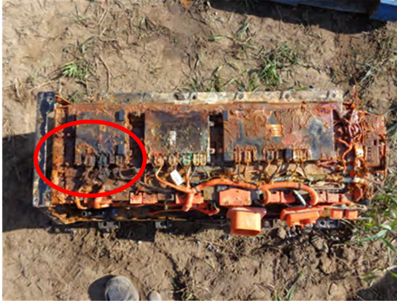
Figure 215 - Ford Focus UP EV post test electronic module connector heat damage.
