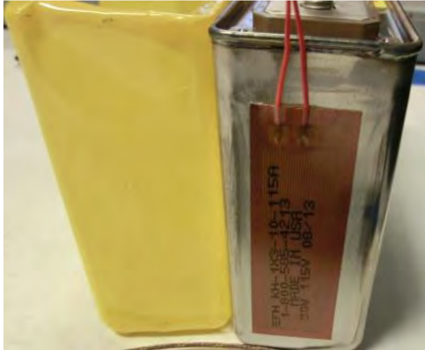
Figure 36 - One of the dual side heater pads.
