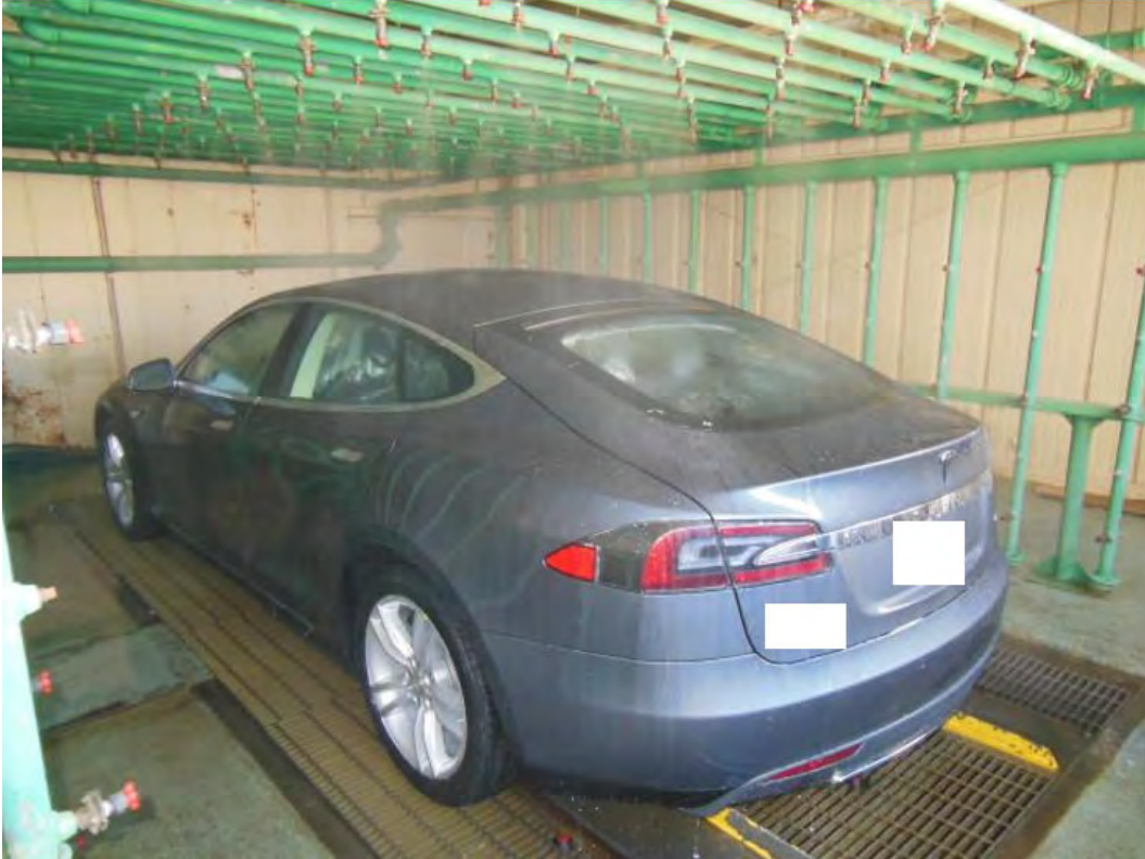
Figure 27 - An example of a vehicle installed in the booth used for rain and drizzle testing. Rain is simulated by applying a total water flow rate of 600 GPM divided into 150 GPM per side (top, left, right, and bottom).
