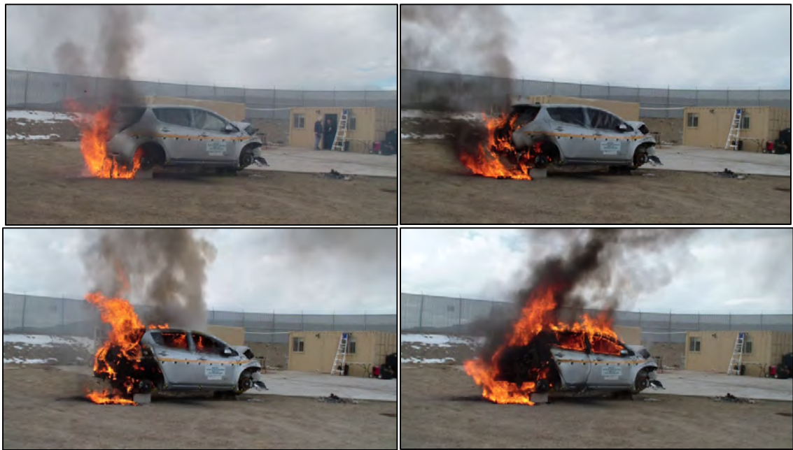
Figure 104 - Top left: 23:41, ignition has occurred. Top right: 26:44, rear flames continue. Bottom left: 28:22, flames inside cabin. Bottom right: 30:53, many internal flames.
