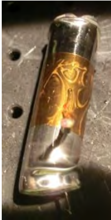
Figure 22 - Cylindrical cell after failed nail penetration trial.
