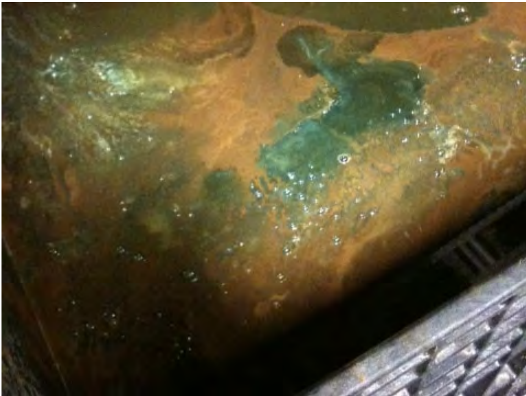
Figure 13 - An example of a salt bath with submerged modules. Note the bubbles of gas on the surface produced by electrolysis.
