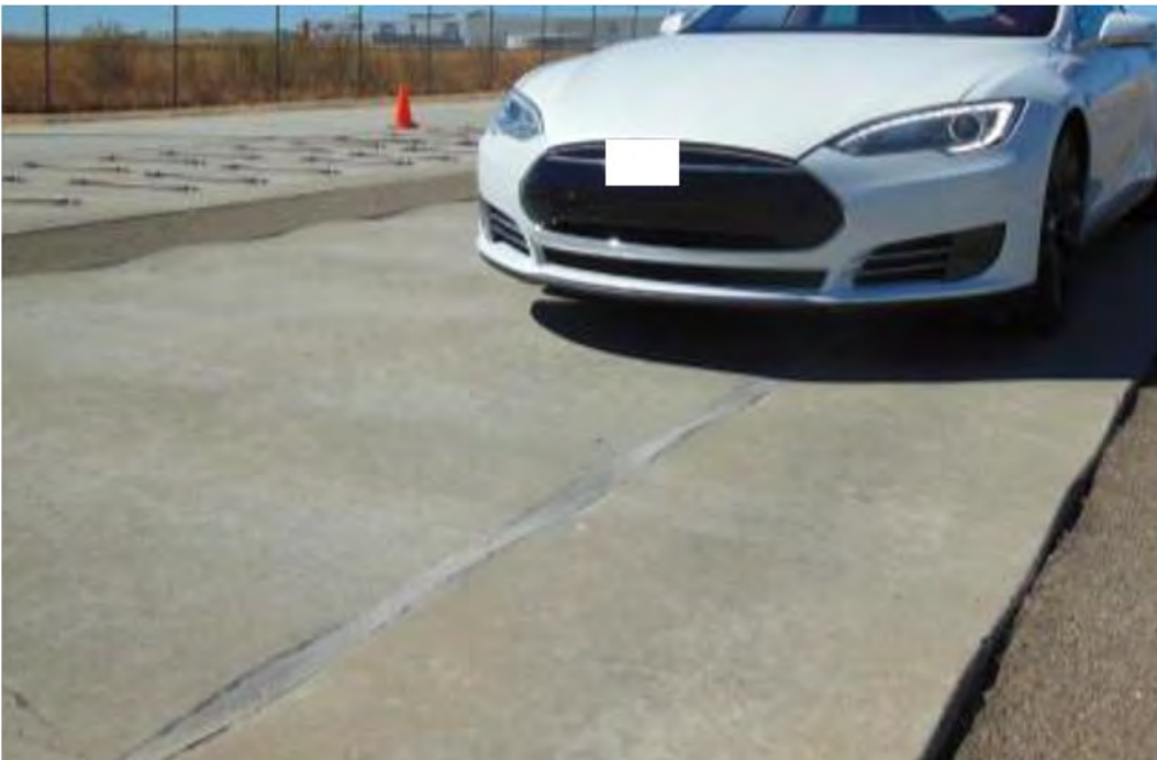
Figure 22 - An example of a vehicle on a wave / sinusoidal road (i.e., rough road element).
