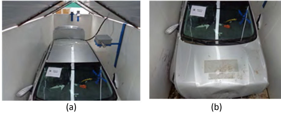
Figure 153 - Hyundai Sonata HEV setup: a) video camera, and b) the vehicle in its immersion container.
