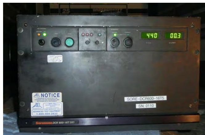
Figure 40 - The Sorenson DCR-600 DC power supply used for both overvoltage and overcurrent overcharge testing. It is rated for 600 V / 16 A (9.6 kW).
