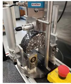
Shaped Compacted Tension (DCT) test and Hamburg Wheel Tracking Test (HWTT) were conducted to evaluate intermediate-temperature cracking resistance, lowtemperature cracking resistance; and rutting and moisture damage resistance, respectively.
