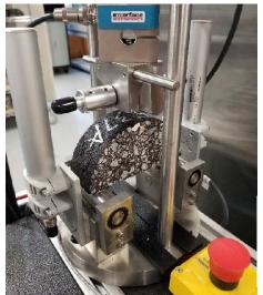
Shaped Compacted Tension (DCT) test and Hamburg Wheel Tracking Test (HWTT) were conducted to evaluate intermediate-temperature cracking resistance, low-temperature cracking resistance; and rutting and moisture damage resistance, respectively.
