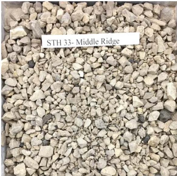
STH 33 – Middle Ridge: Crushed aggregate of sedimentary origin (carbonates: dolostone/limestone). Angular and semi-angular particles with rough surface texture.
