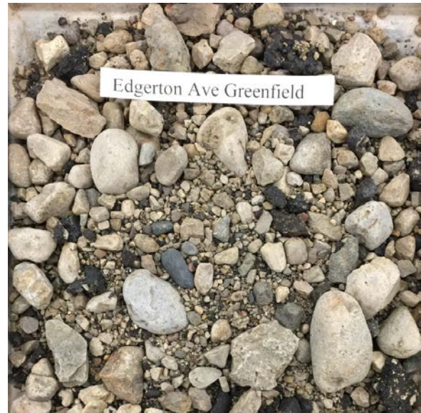
Edgerton Ave. – Greenfield: Natural gravel of sedimentary origin (carbonates: limestone/dolostone) with a lesser amount of particles of igneous and metamorphic origin. Semi-round particles, a large percentage with smooth surface texture; some crushed particles with semi-angular shape.
