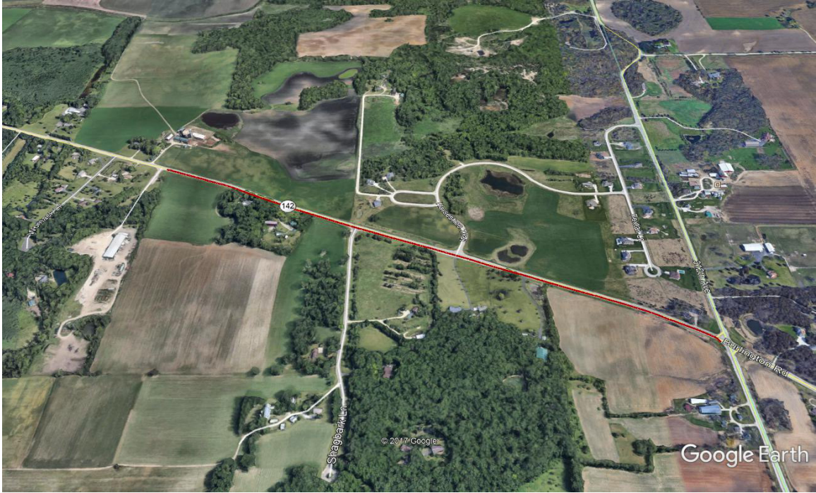
(a) Track of the GPR testing at STH 142 East of Burlington: outside wheel path of the eastbound (left to right in the picture)
