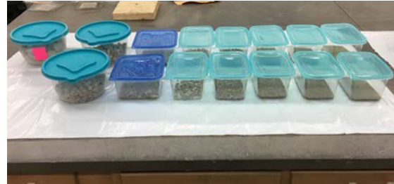
(b) Aggregate specimens prepared for sodium sulfate test
