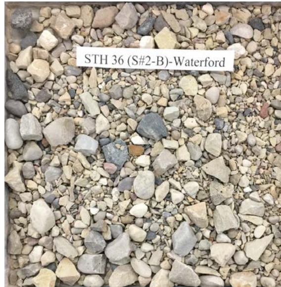
STH 36 Site #2 – Brown: Natural gravel of mixed origin but mainly sedimentary (carbonates: limestone/dolostone). Presence of crushed gravel composed of semi-round particles with smooth surface texture. Some semi-angular particles with rough surface texture present.
