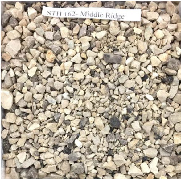
STH 162 – Middle Ridge: Crushed aggregate of sedimentary origin (carbonates: dolostone/limestone). Angular and semi-angular particles with rough surface texture.
