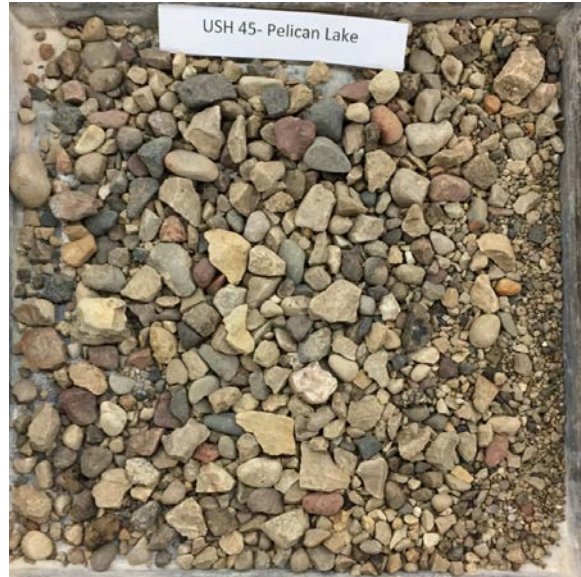
USH 45 – Pelican Lake: Natural gravel of mixed origin: igneous, metamorphic and sedimentary (carbonates). Round and semi round particle shape and smooth surface texture; some crushed gravel particles with semi-angular/angular shape and rough surface texture.
