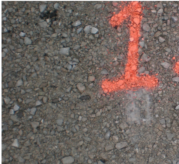
CTH JJ – Appleton: Crushed aggregate of sedimentary origin (carbonates: dolostone/limestone). Angular and semi-angular particles with rough surface texture.
