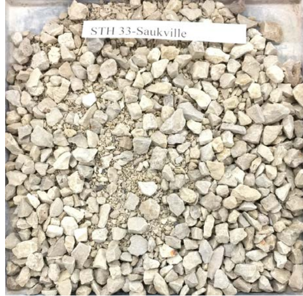
STH 33 – Saukville: Crushed aggregate of sedimentary origin (carbonates: dolostone/limestone). Angular and semi-angular particles with rough surface texture.
