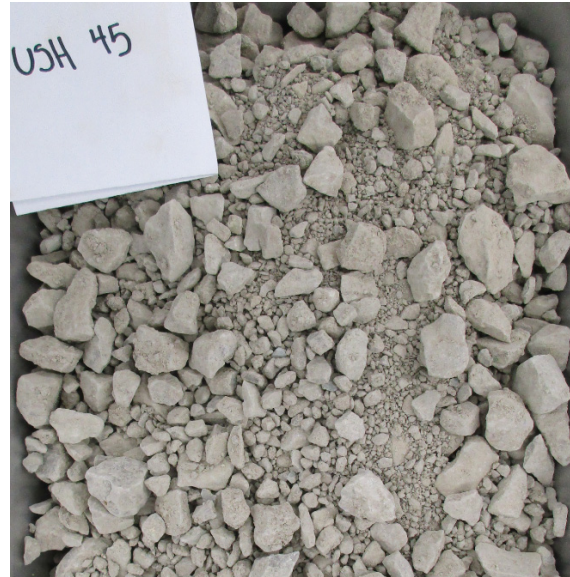
USH 45 – Larsen: Crushed aggregate of sedimentary origin (carbonates: dolostone/ limestone). Angular and semi-angular particles with rough surface texture.
