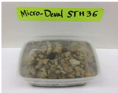
(c) Soaking Micro-Deval test specimen
