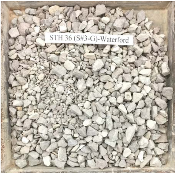
STH 36 Site #3 – Gray: Crushed aggregate of sedimentary origin (carbonates: dolostone/limestone). Angular and semi-angular particles with rough surface texture.
