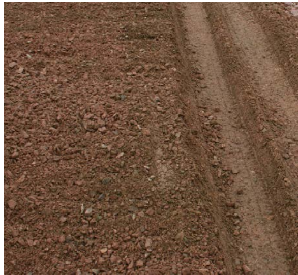
STH 13 – Spencer: Crushed aggregate of igneous and metamorphic origin. Angular and semi-angular particles with rough surface texture.
