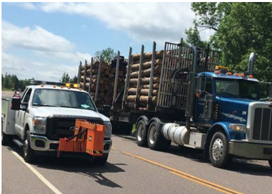
(e) The 2 GHz GPR antenna
