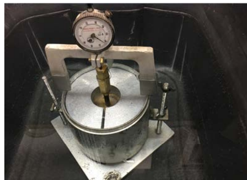
(b) Soaking CBR test specimen
