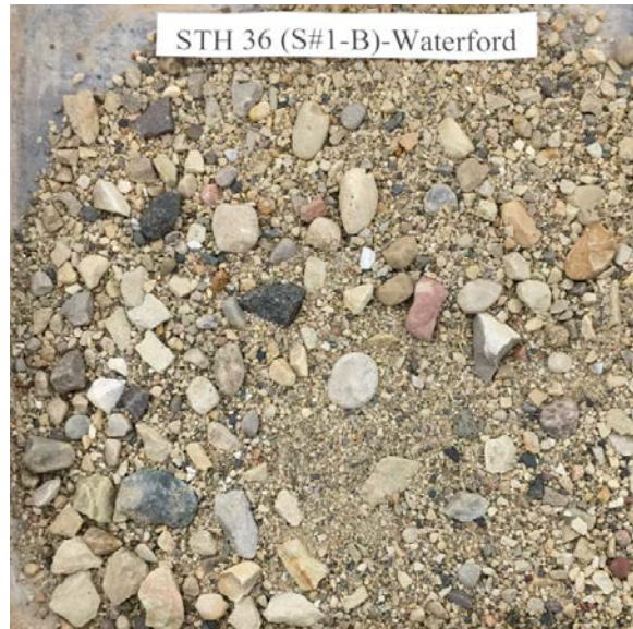
STH 36 Site #1 – Brown: Natural gravel of mixed origin but mainly sedimentary (carbonates: limestone/dolostone). Presence of crushed gravel composed of semi-round particles with smooth surface texture. Some semi-angular particles with rough surface texture present.
