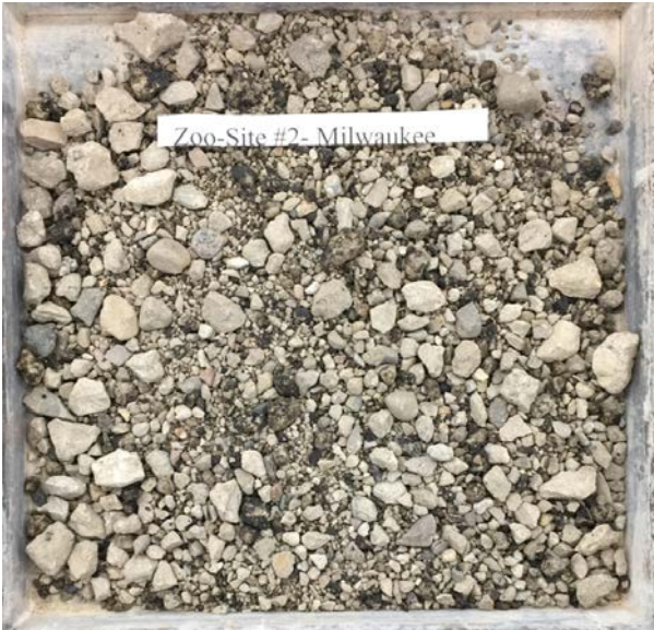
I 94 – Zoo Interchange Site #2: Mixture of crushed aggregate of sedimentary origin (carbonates: limestone/dolostone) with smaller percentages of recycled crushed Portland cement concrete (RC) and recycled asphalt pavement (RAP). Angular/semi-angular particles with rough surface texture and noticeable porosity.
