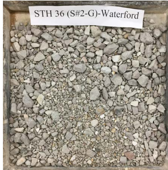
STH 36 Site #2 – Gray: Crushed aggregate of sedimentary origin (carbonates: dolostone/limestone). Angular and semi-angular particles with rough surface texture.
