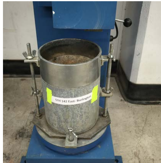
(b) Compacting aggregate samples
