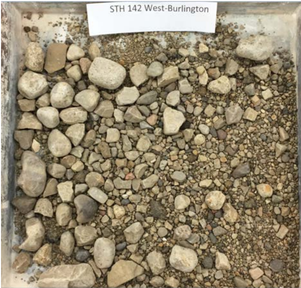
STH 142 West – Burlington: Natural gravel of sedimentary origin (carbonates: limestone/ dolostone). Round and semi-round particles, a large percentage with smooth surface texture; some crushed particles with semi-angular shape. Presence of large sized particles.
