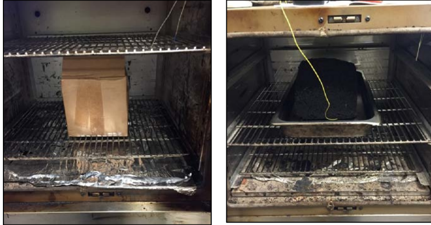
Figure 3. Reheating Boxed versus Unboxed HMA Blocks.
