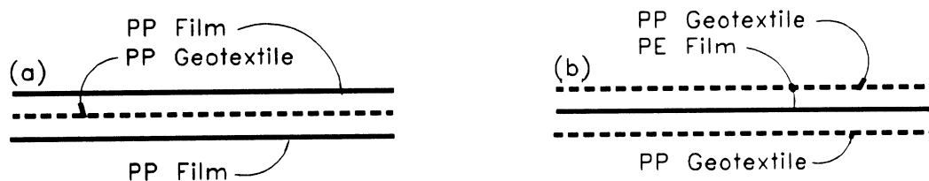
Figure 10-1 Thin-film geotextile composites: (a) PP film / PP geotextile / PP film; and (b) PP geotextile - PE film - PP geotextile.
