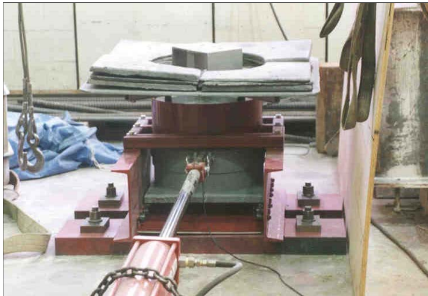
Figure 1. Large-scale direct shear testing device.
