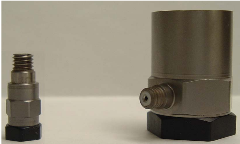
Figure 3.4 Accelerometers used for SASW tests. Model 352C68 shown at left, model 353B33 shown at right.
