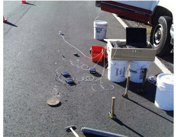
Figure 3.13 SASW equipment setup at Beulah test site
