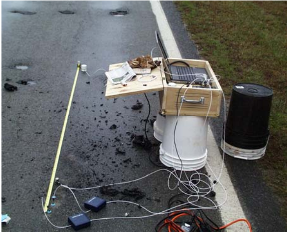
Figure 3.12 SASW equipment setup at Hot Springs site
