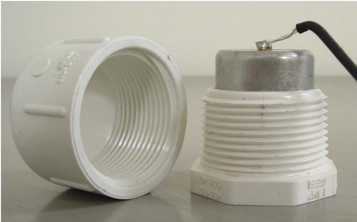
Figure 3.5 L-28V geophone shown inside a PVC housing. A soldered wire lead is connected to the top of the geophone
