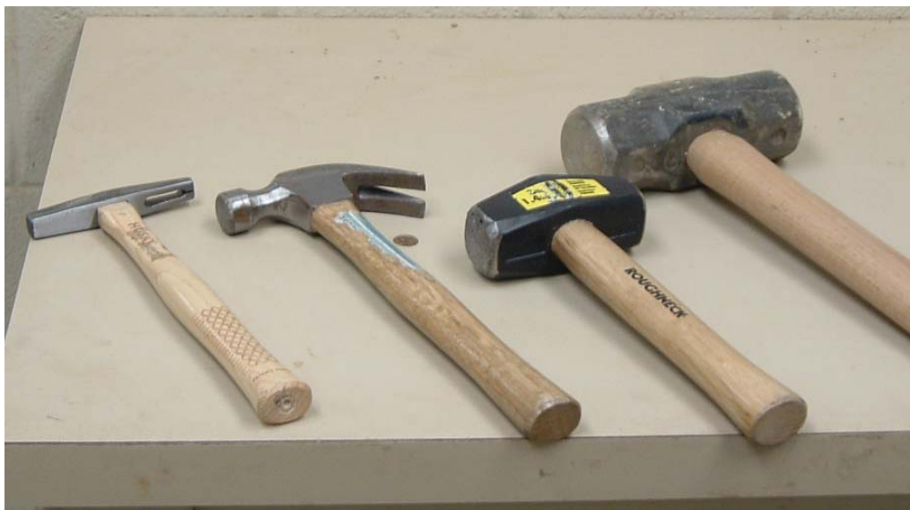
Figure 3.2 Sources used during SASW testing. From left to right: tack hammer, claw hammer, 3 lb sledge hammer, 8 lb sledge hammer
