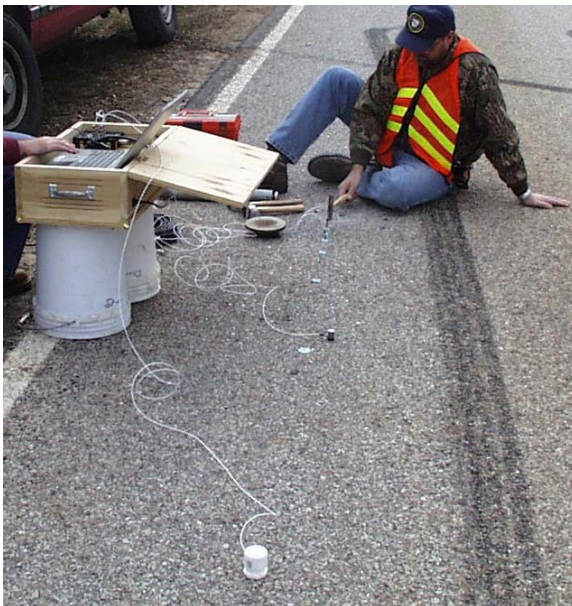
Figure 3.10 SASW test setup at Mountain Home
