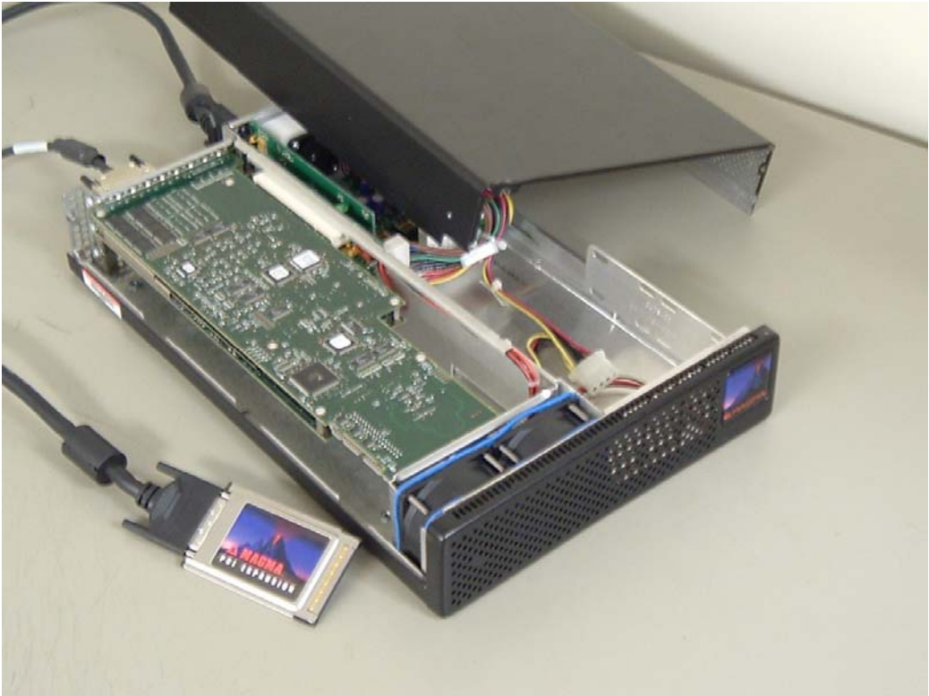
Figure 3.7 NI-4552 digital signal analyzer mounted in PCI expansion chassis
