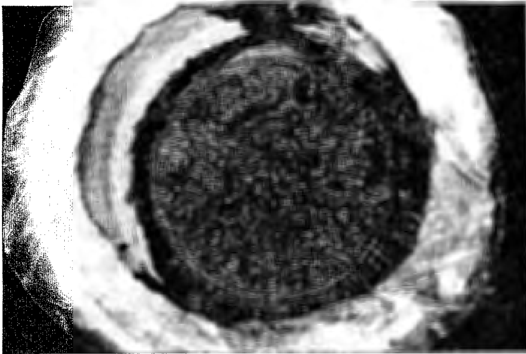
Figure 6.31: Wisconsin Silty Clay Till Specimen Surface Underlying 1101 Geotextile
